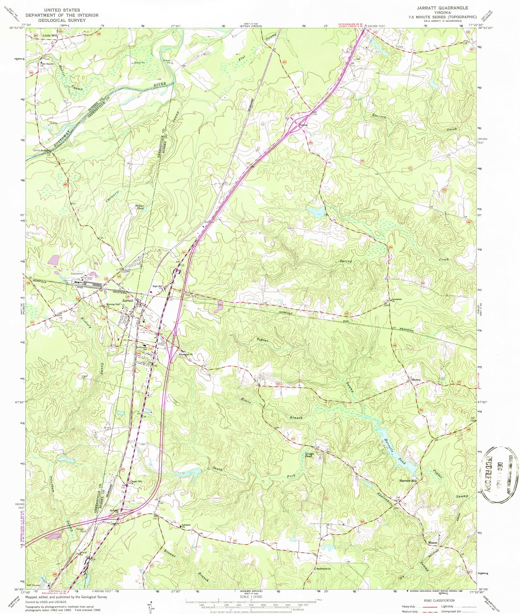
Polyconic projection. 1927 North American datum 10,000-foot grid based on Virginia coordinate system, south zone 1000-meter Universal Transverse Mercator grid ticks, zone 18, shown in blue
