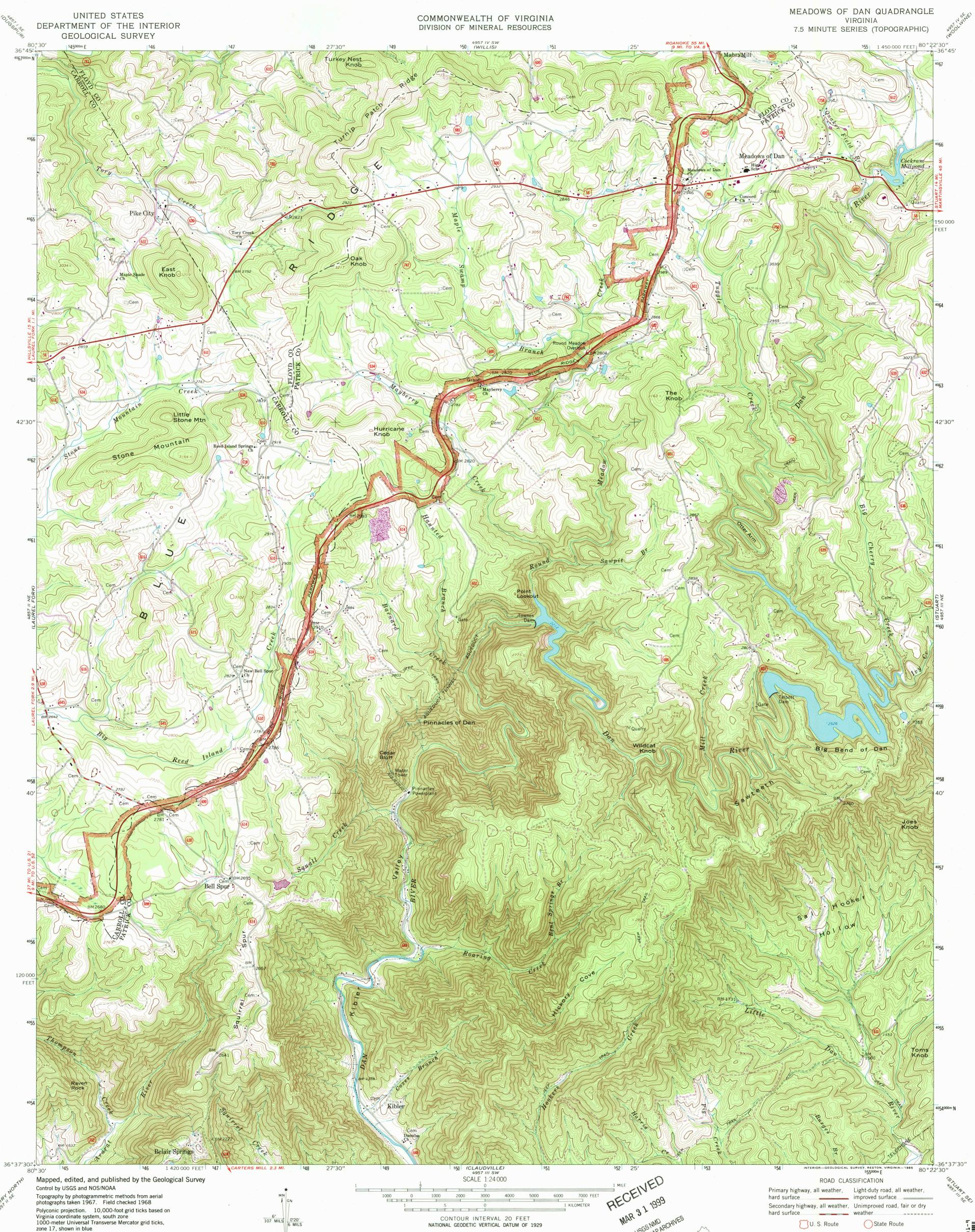
Polyconic projection. 10,000-foot grid ticks based on Virginia coordinate system, south zone 1000-meter Universal Transverse Mercator grid ticks, zone 17, shown in blue 1927 North American Datum To place on the predicted North American Datum 1983 move the projection lines 9 meters south and 18 meters west as shown by dashed corner ticks
