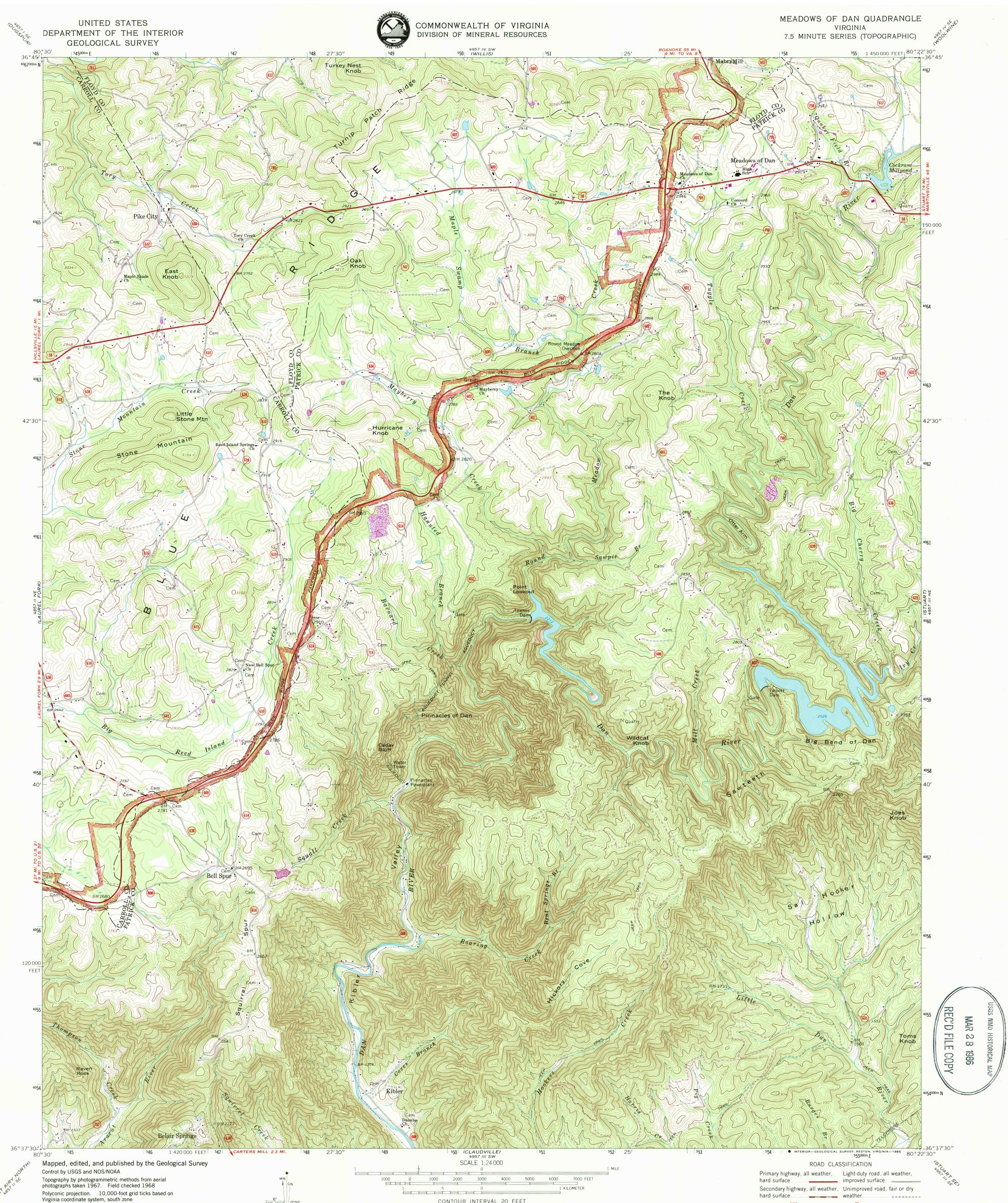
1000-meter Universal Transverse Mercator grid ticks, zone 17, shown in blue 1927 North American Datum To place on the predicted North American Datum 1983 move the projection lines 9 meters south and 18 meters west as shown by dashed corner ticks
