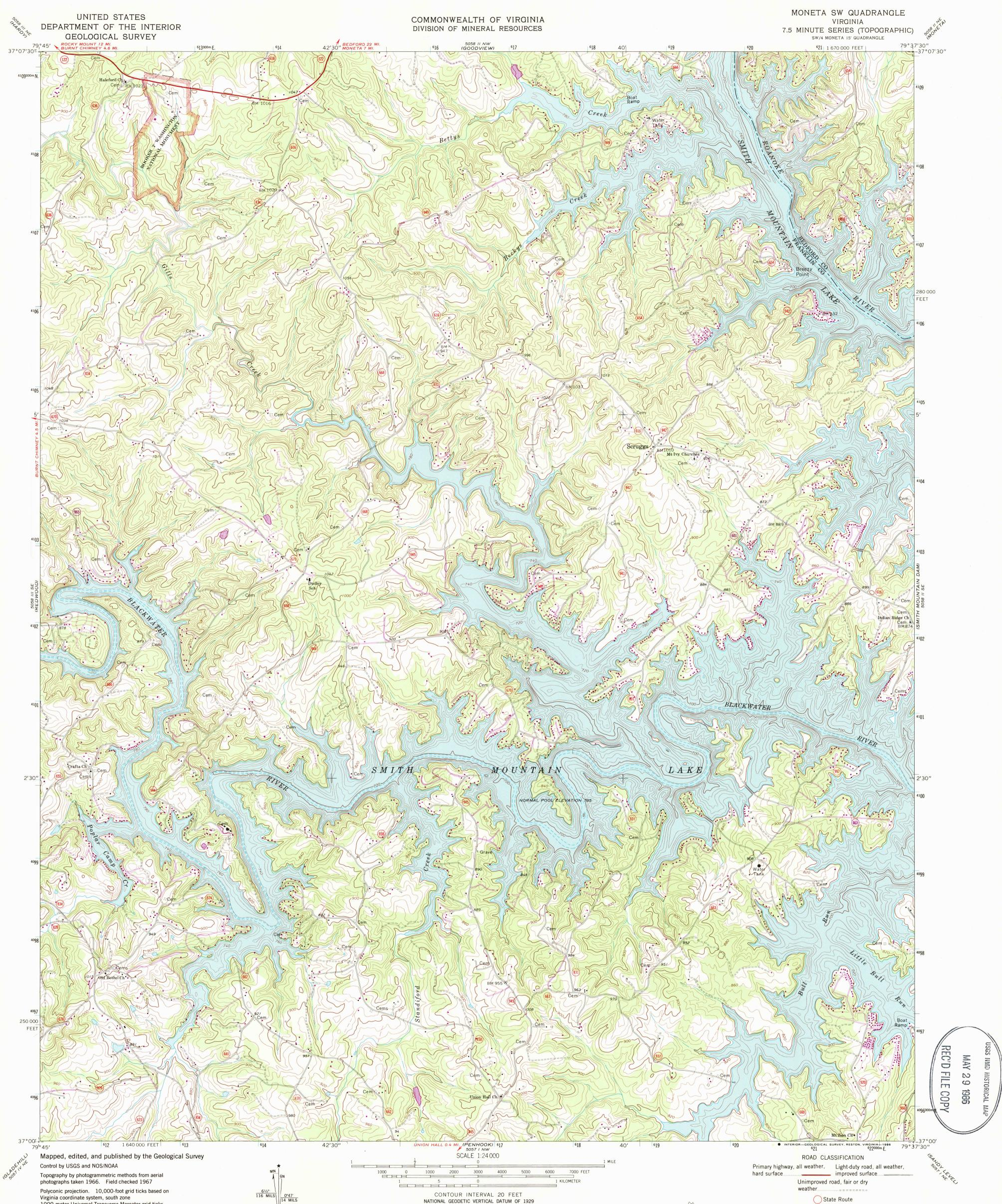
Polyconic projection. 10,000-foot grid ticks based on Virginia coordinate system, south zone 1000-meter Universal Transverse Mercator grid ticks, zone 17, shown in blue 1927 North American Datum To place on the predicted North American Datum 1983 move the projection lines 10 meters south and 20 meters west as shown by dashed corner ticks Fine red dashed lines indicate selected fence and field lines where generally visible on aerial photographs. This information is unchecked
