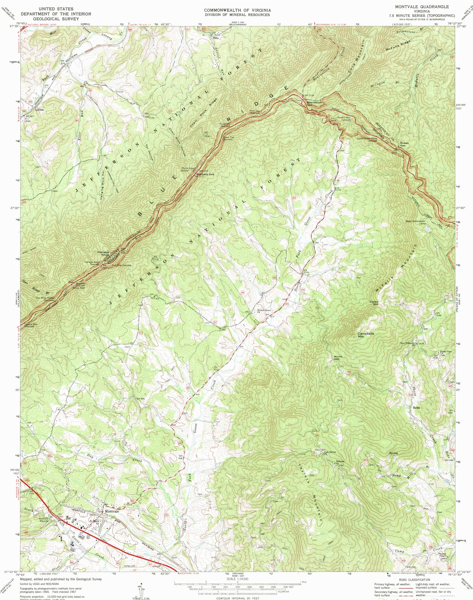
Virginia coordinate system, south zone 1000-meter Universal Transverse Mercator grid ticks, zone 17, shown in blue. 1927 North American Datum To place on the predicted North American Datum 1983 move the projection lines 10 meters south and 20 meters west as shown by dashed corner ticks
