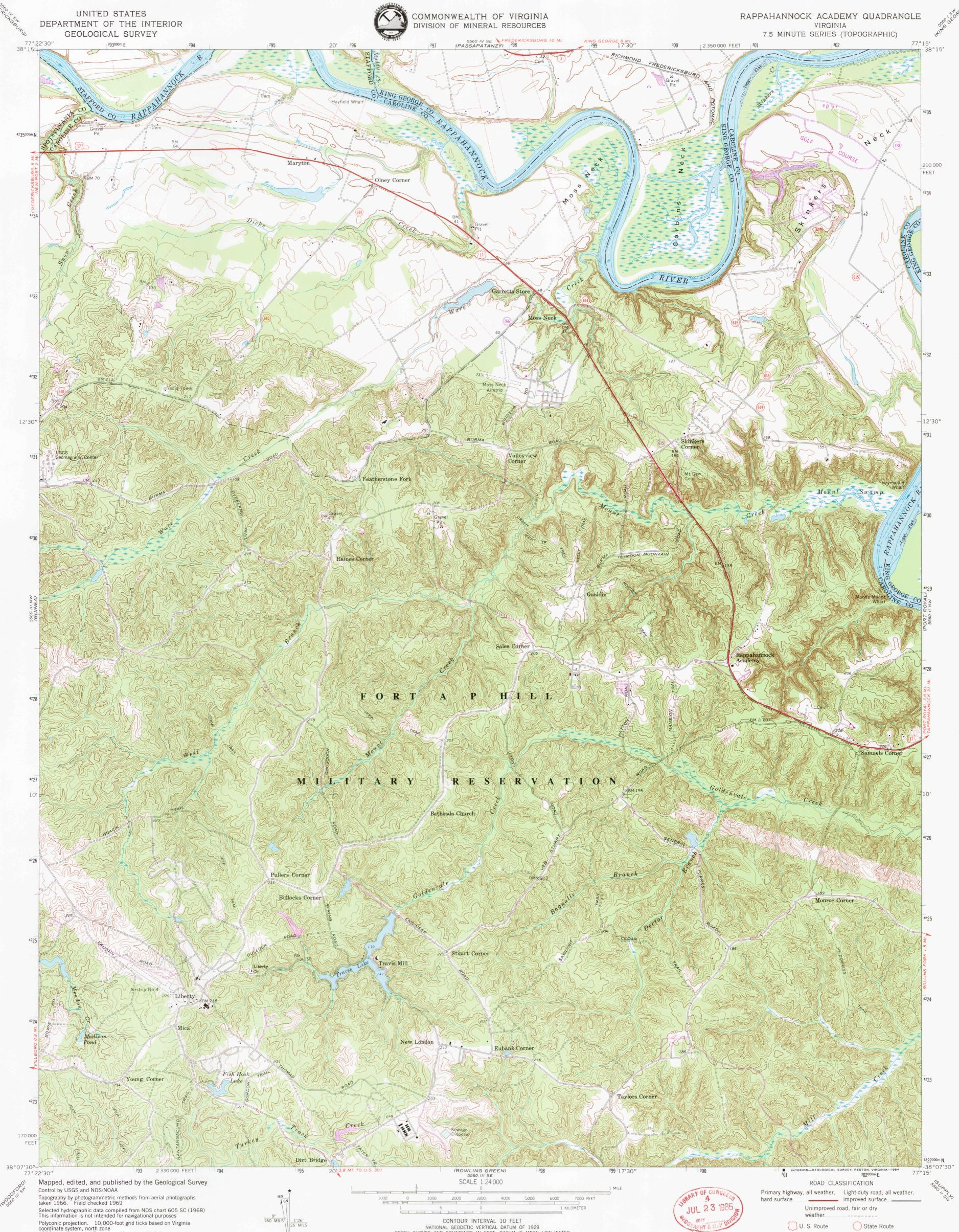
coordinate system, north zone 1000-meter Universal Transverse Mercator grid ticks, zone 18, shown in blue 1927 North American Datum To place on the predicted North American Datum 1983 move the projection lines 10 meters south and 26 meters west as shown by dashed corner ticks
