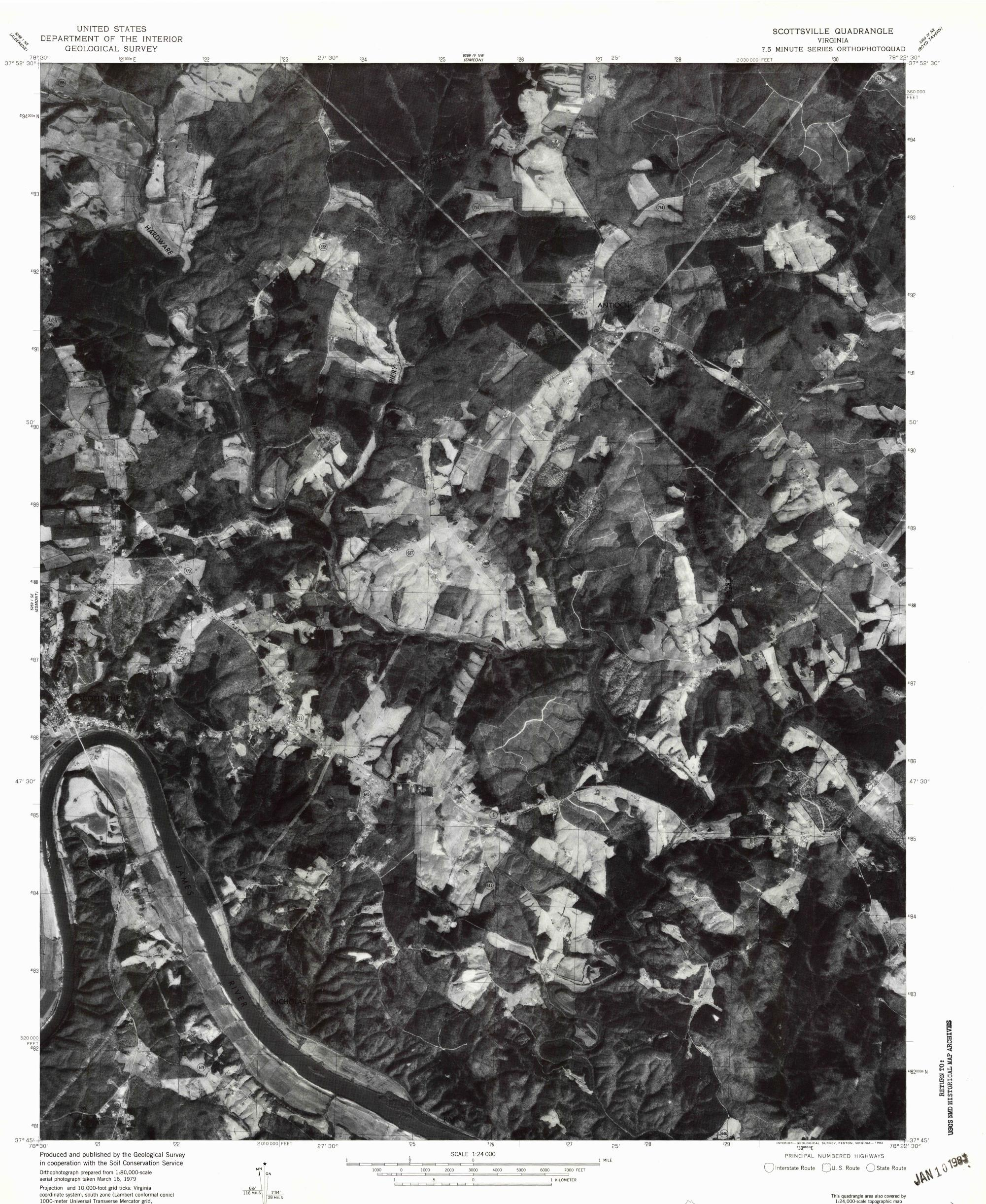
Projection and 10,000-foot grid ticks: Virginia coordinate system, south zone (Lambert conformal conic) 1000-meter Universal Transverse Mercator grid, zone 17. 1927 North American Datum
