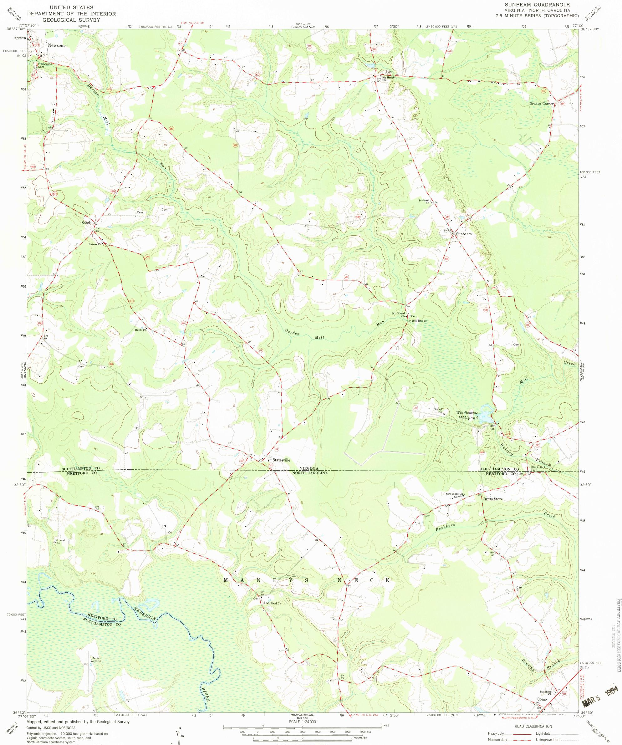
1000-meter Universal Transverse Mercator grid ticks zone 18, shown in blue. 1927 North American Datum To place on the predicted North American Datum 1983 move the projection lines 12 meters south and 28 meters west as shown by dashed corner ticks
