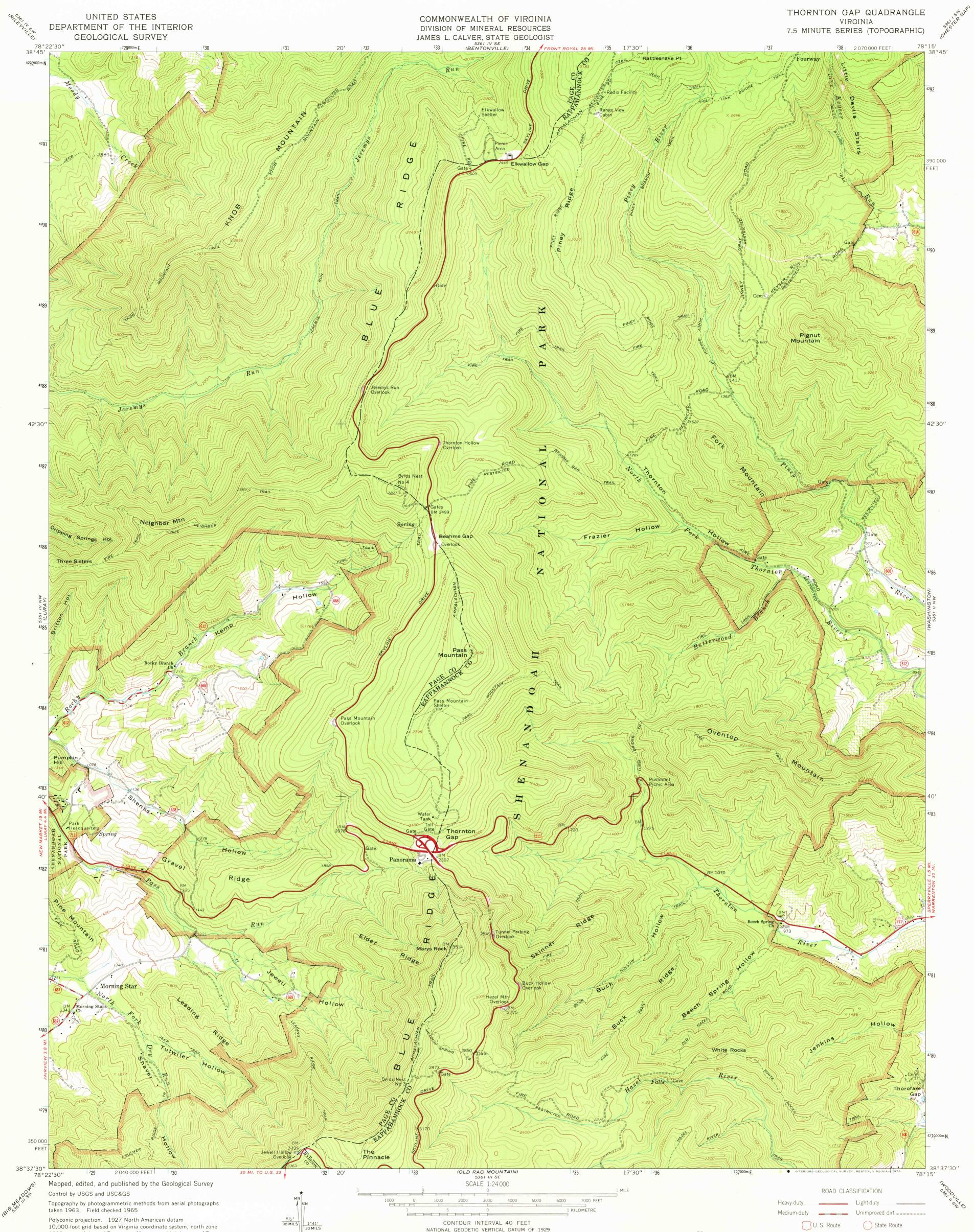
Polyconic projection. 1927 North American datum 10,000-foot grid based on Virginia coordinate system, north zone 1000-metre Universal Transverse Mercator grid ticks, zone 17, shown in blue
