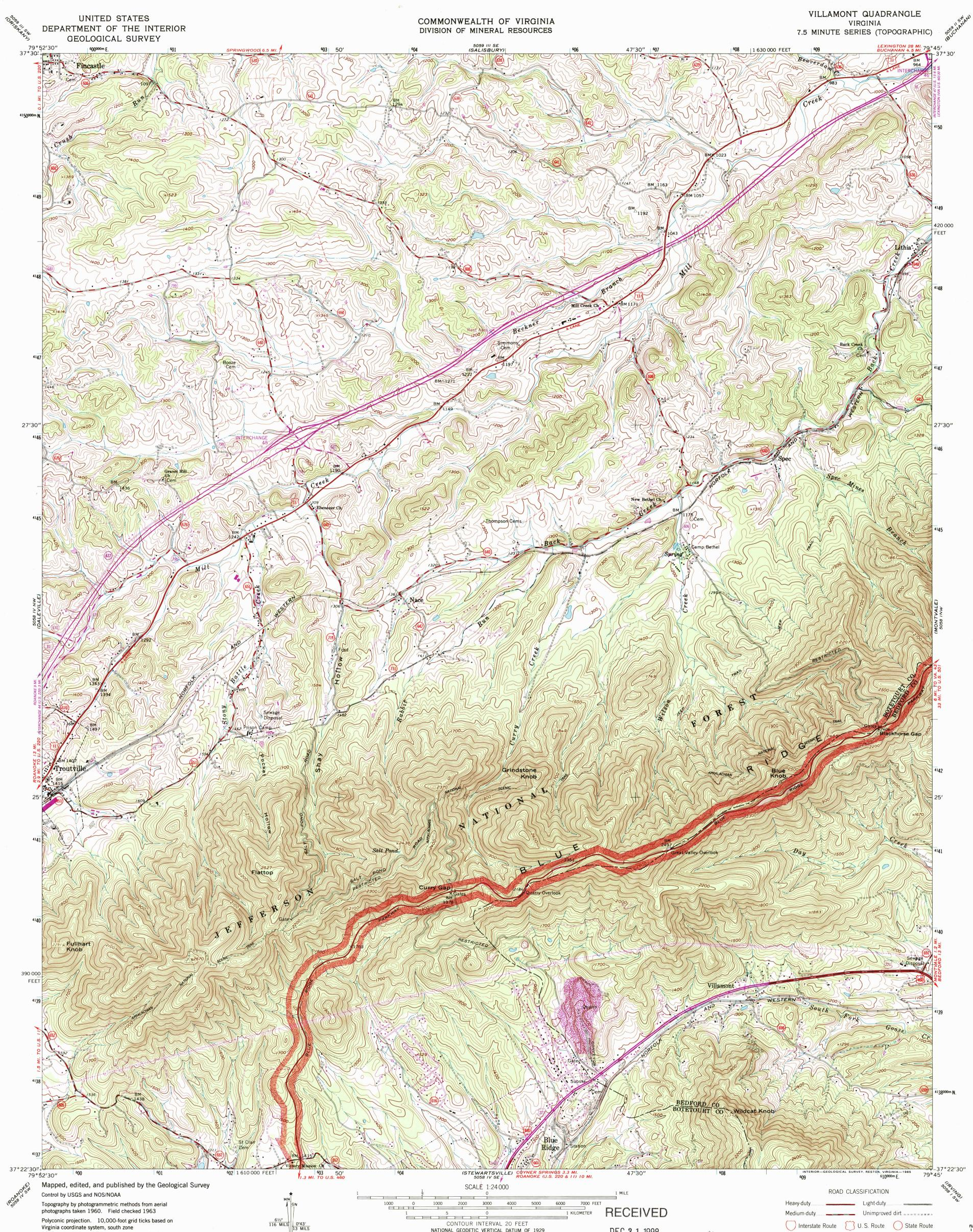
Polyconic projection. 10,000-foot grid ticks based on Virginia coordinate system, south zone 1000-meter Universal Transverse Mercator grid ticks, zone 17, shown in blue 1927 North American Datum To place on the predicted North American Datum 1983 move the projection lines 10 meters south and 20 meters west as shown by dashed corner ticks
