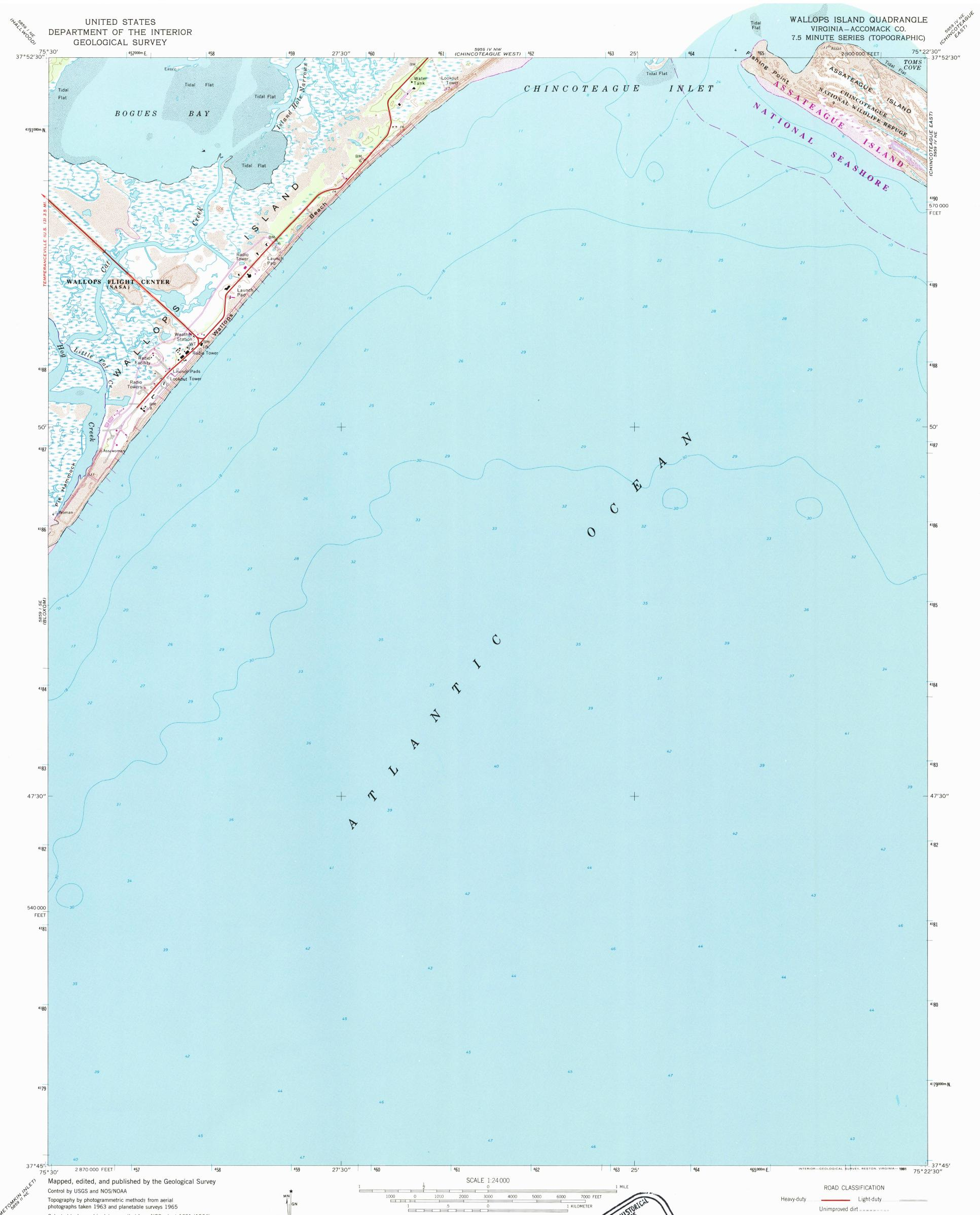
Selected hydrographic data compiled from NOS chart 1221 (1964) This information is not intended for navigational purposes Polyconic projection. 10,000-foot grid based on Virginia coordinate system, south zone 1000-meter Universal Transverse Mercator grid ticks, zone 18, shown in blue. 1927 North American Datum To place on the predicted North American Datum 1983 move the projection lines 9 meters south and 31 meters west as shown by dashed corner ticks
