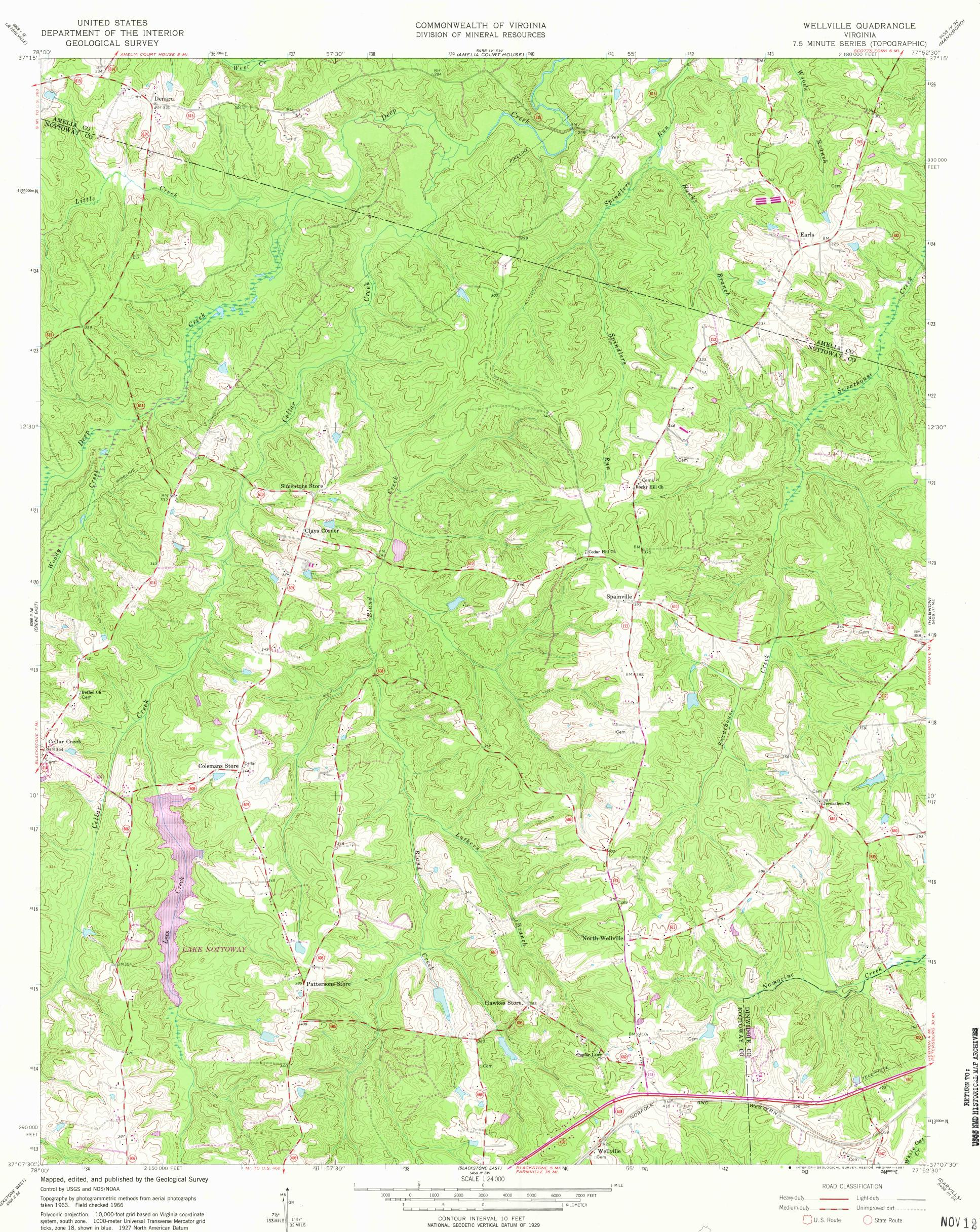
Polyconic projection. 10,000-foot grid based on Virginia coordinate system, south zone. 1000-meter Universal Transverse Mercator grid ticks, zone 18, shown in blue. 1927 North American Datum To place on the predicted North American Datum 1983 move the projection lines 12 meters south and 26 meters west as shown by dashed corner ticks
