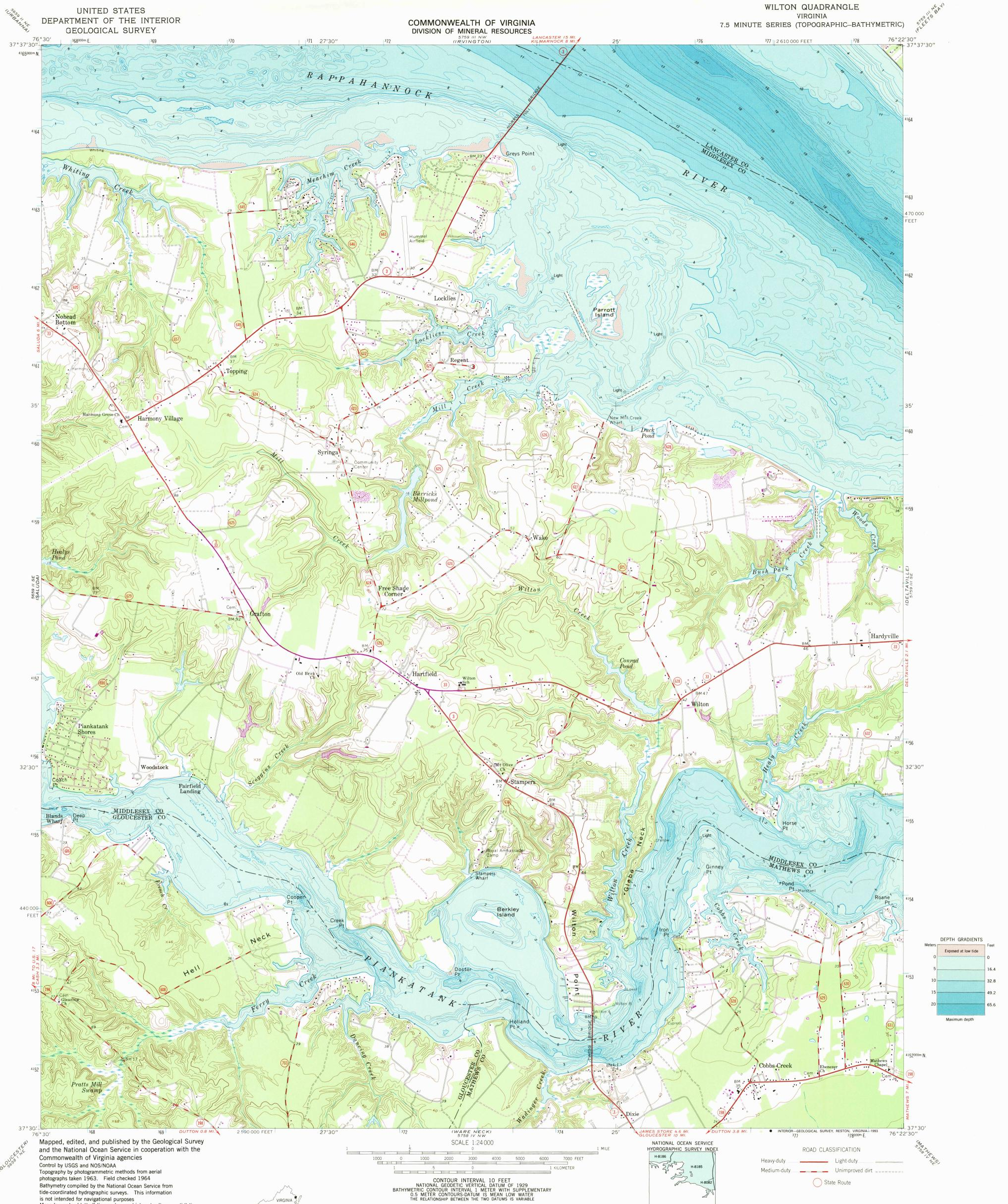
Bathymetry compiled by the National Ocean Service from tide-coordinated hydrographic surveys. This information is not intended for navigational purposes Mean low water (dotted) line and mean high water (heavy solid) line compiled by NOS from tide-coordinated aerial photographs Apparent shoreline (outer edge of vegetation) shown by light solid line Polyconic projection. 1927 North American Datum 10,000-foot grid based on Virginia coordinate system, south zone
