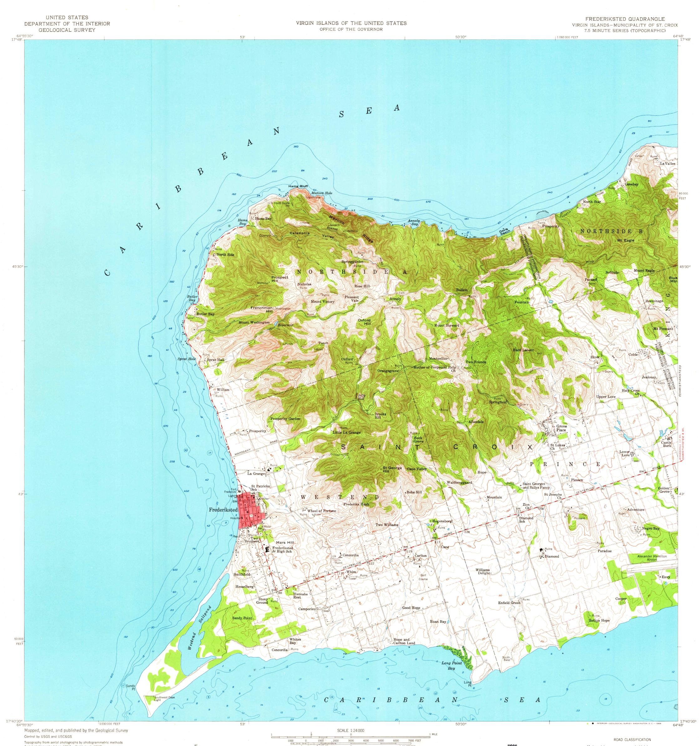
Topography from aerial photographs by photogrammetric methods Aerial photographs taken 1954. Field check 1958 Hydrography compiled from USC&GS charts 905 and 937 (1952) Polyconic projection. Puerto Rican datum, 1940 adjustment 10,000-foot grid based on Puerto Rican coordinate system, Puerto Rico, St. Croix zone Fine red dashed lines indicate selected fence and field lines visible on aerial photographs. This information is unchecked
