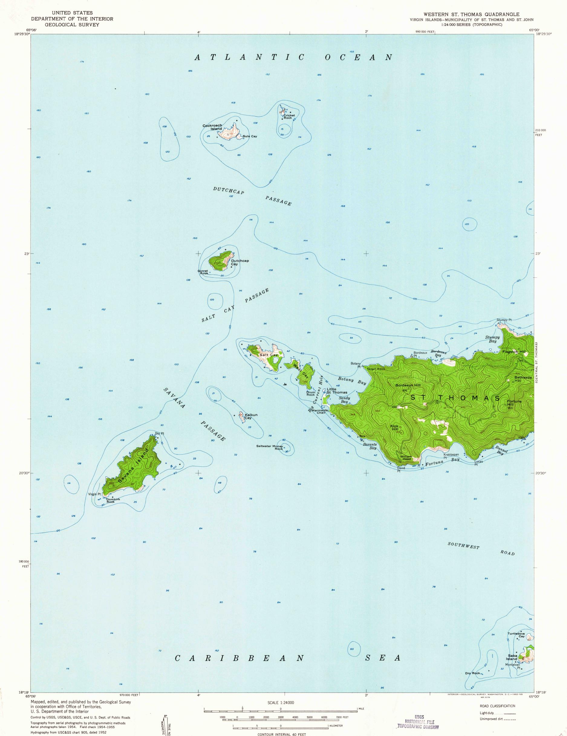
Hydrography from USC&GS chart 905, dated 1952 Folyconic projection. Puerto Rican datum, 1940 adjustment 10,000-foot grid based on Puerto Rican coordinate system, Virgin Islands extension Unchecked elevations are shown in brown
