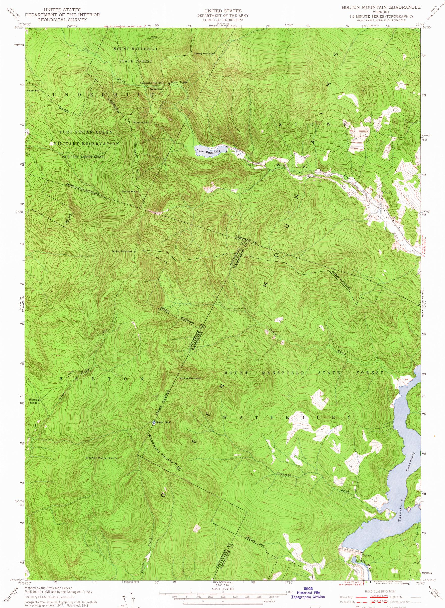
Aerial photographs taken 1947. Field check 1948 Polyconic projection. 1927 North American datum 10,000-foot grid based on Vermont coordinate system No distinction is made between barns, dwellings, commercial and industrial buildings Unchecked elevations are shown in brown The Long Trail shown in approximate location 1000-meter Universal Transverse Mercator grid ticks, zone 18, shown in blue
