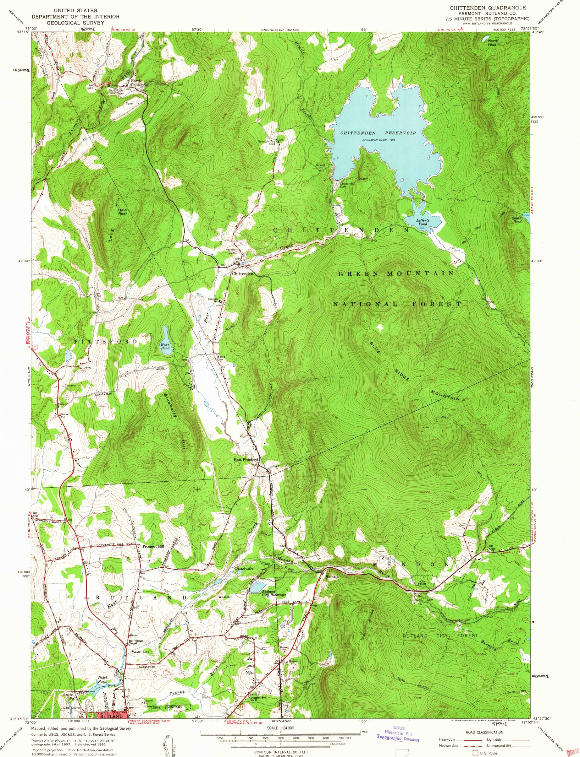
Polyconic projection. 1927 North American datum 10,000-foot grid based on Vermont coordinate system 1000-meter Universal Transverse Mercator grid ticks, zone 18, shown in blue
