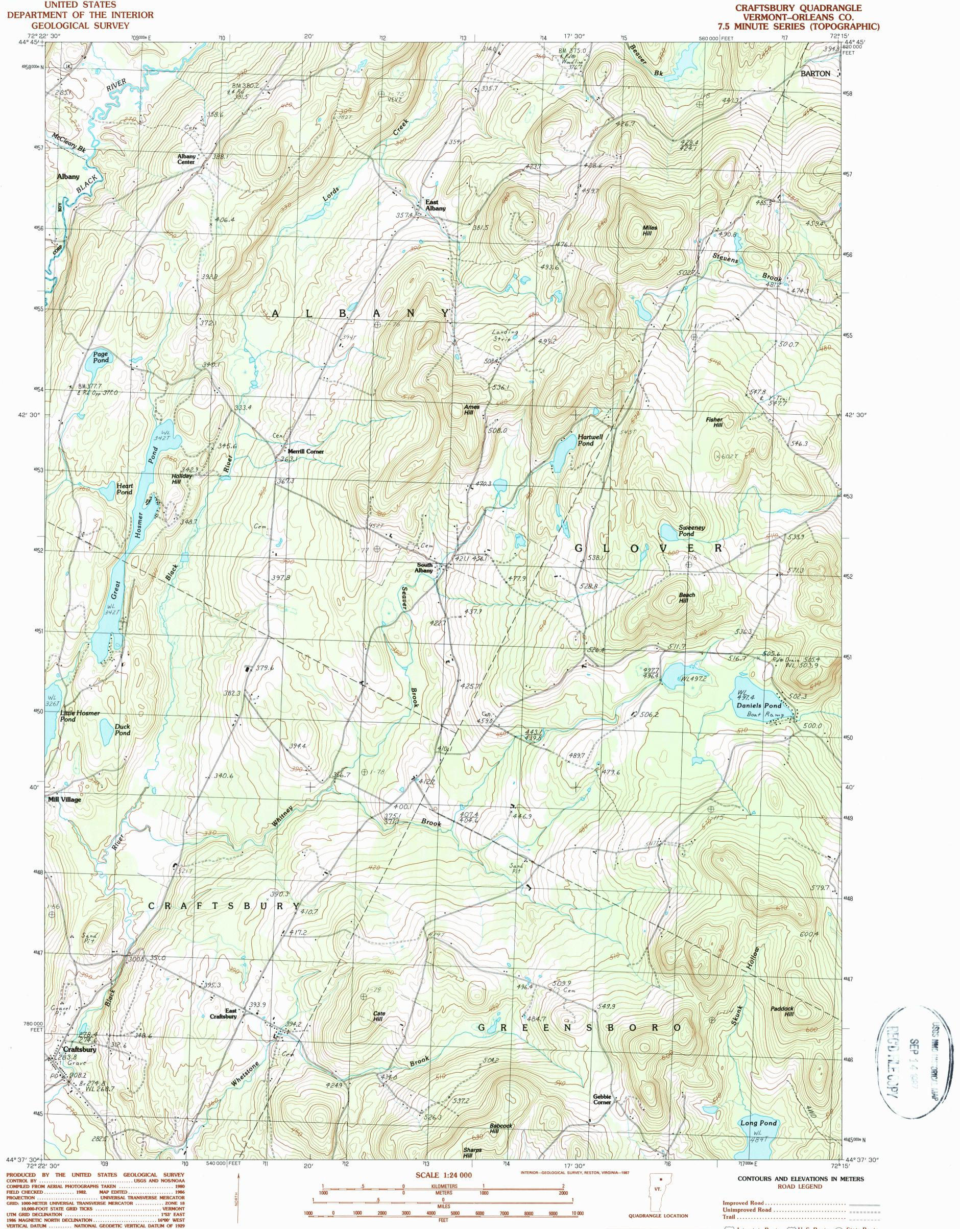
CONTOUR INTERVAL 6 METERS CONTROL AND FIELD ESTABLISHED ELEVATIONS SHOWN TO THE NEAREST 0.1 METER OTHER ELEVATIONS SHOWN TO THE NEAREST METER To convert meters to feet multiply by 3.2808 To convert feet to meters multiply by .3048 THIS MAP COMPLIES WITH NATIONAL MAP ACCURACY STANDARDS FOR SALE BY U. S. GEOLOGICAL SURVEY DENVER, COLORADO 80225, OR RESTON, VIRGINIA 22092
