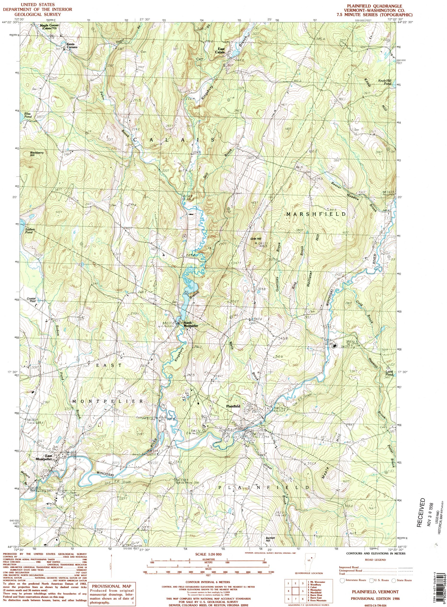
UTM GRID DECLINATION ..... VERTICAL DATUM ..... NATIONAL GEODETIC VERTICAL DATUM OF 1929 HORIZONTAL DATUM ...... 1927 NORTH AMERICAN DATUM To place on the predicted North American Datum of 1983, move the projection lines as shown by dashed corner ticks (2 meters south and 36 meters west) There may be private inholdings within the boundaries of any Federal and State reservations shown on this map No distinction made between houses, barns, and other buildings
