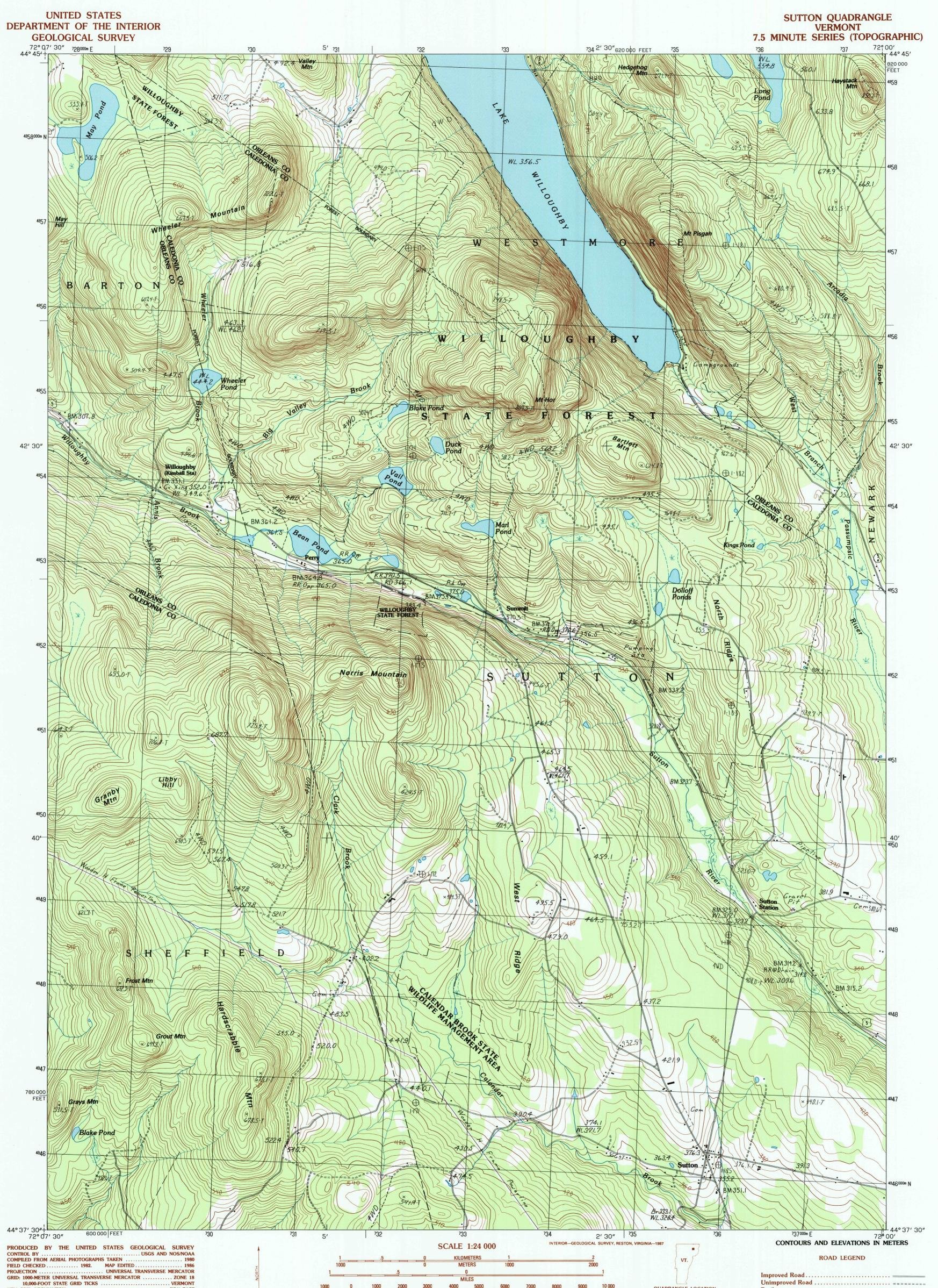
10,000-FOOT STATE GRID TICKS ..... VERMONT VERTICAL DATUM ...... NATIONAL GEODETIC VERTICAL DATUM OF 1929 HORIZONTAL DATUM ...... 1927 NORTH AMERICAN DATUM To place on the predicted North American Datum of 1983, move the projection lines as shown by dashed corner ticks (2 meters south and 37 meters west) There may be private inholdings within the boundaries of any Federal and State reservations shown on this map No distinction made between houses, barns, and other buildings
