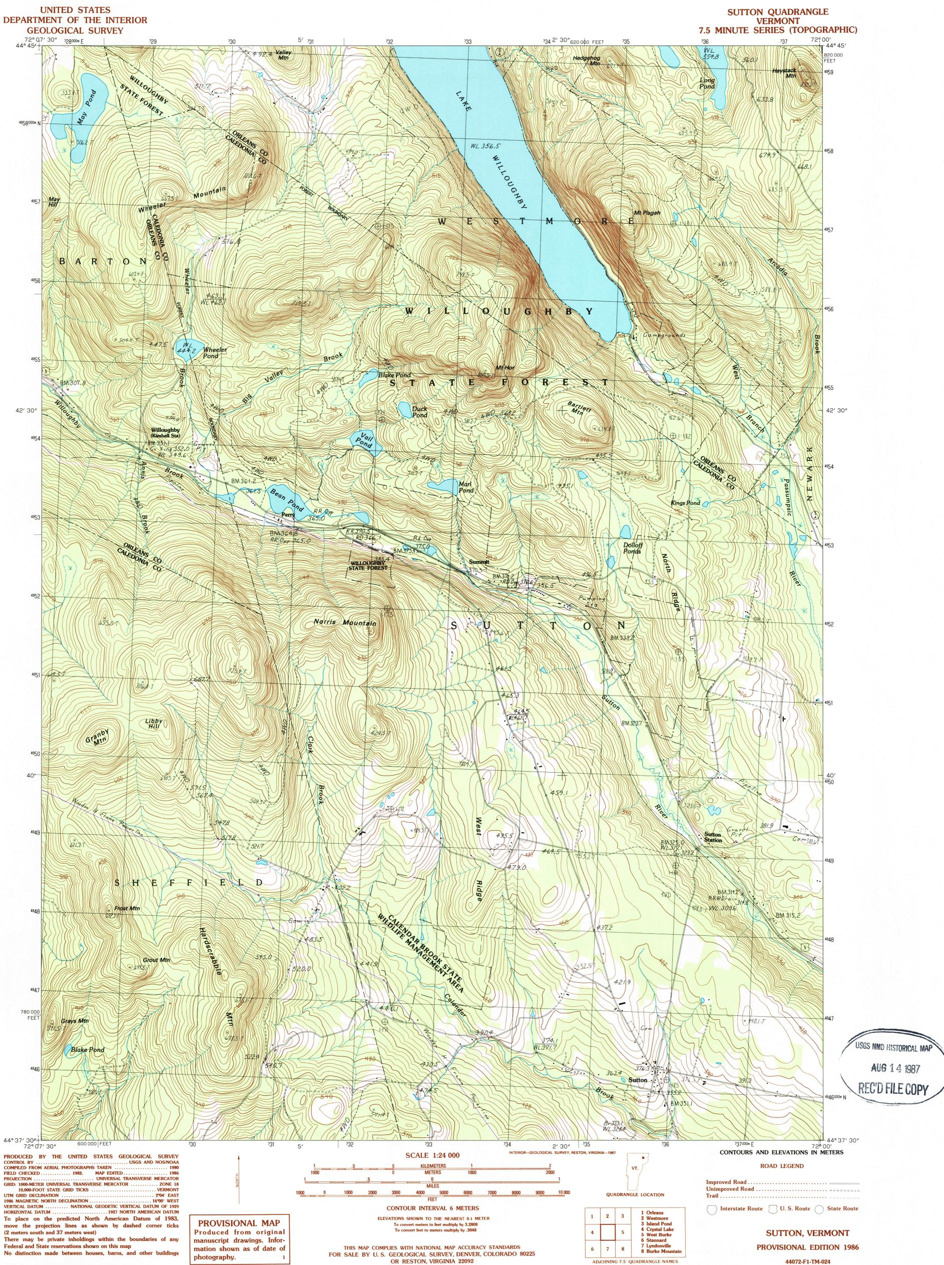
VERTICAL DATUM ...... NATIONAL GEODETIC VERTICAL DATUM OF 1929 HORIZONTAL DATUM ...... 1927 NORTH AMERICAN DATUM To place on the predicted North American Datum of 1983, move the projection lines as shown by dashed corner ticks (2 meters south and 37 meters west) There may be private inholdings within the boundaries of any Federal and State reservations shown on this map No distinction made between houses, barns, and other buildings
