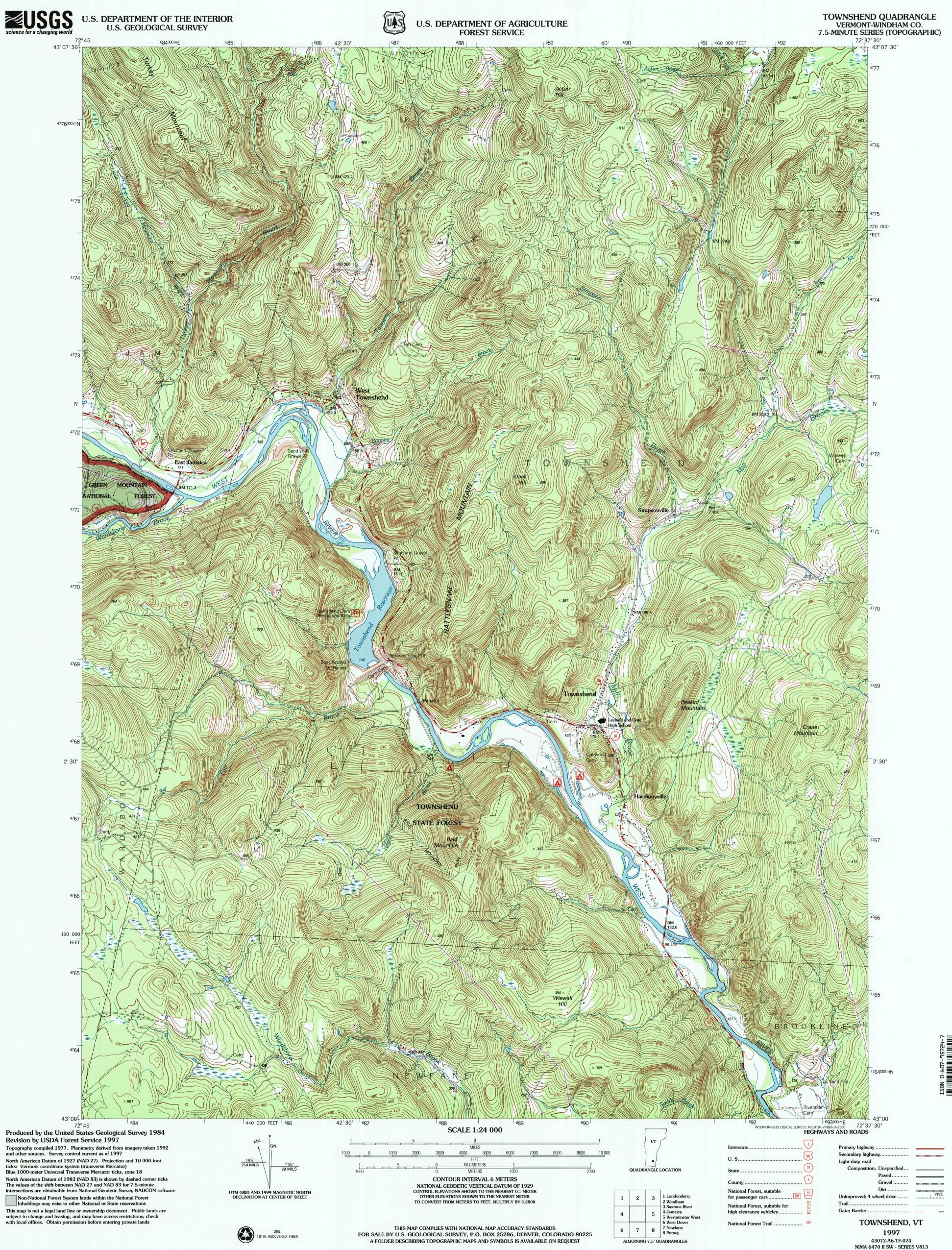
Blue 1000-meter Universal Transverse Mercator ticks, zone 18 North American Datum of 1983 (NAD 83) is shown by dashed corner ticks The values of the shift between NAD 27 and NAD 83 for 7.5-minute intersections are obtainable from National Geodetic Survey NADCON software
