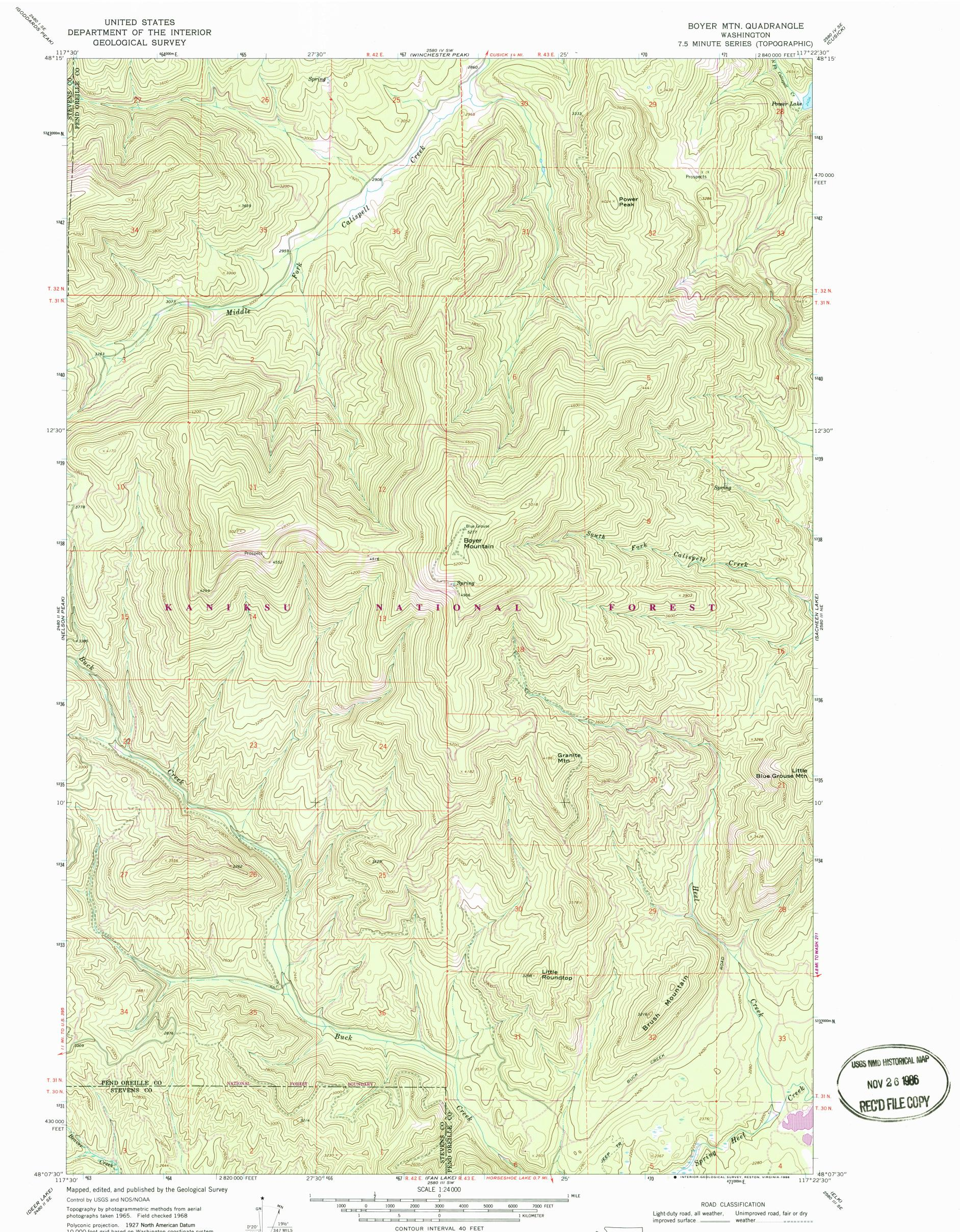
Polyconic projection. 1927 North American Datum 10,000-foot grid based on Washington coordinate system, 6 MILS north zone 1000-meter Universal Transverse Mercator grid ticks, zone 11, shown in blue UTM GRID AND 1986 MAGNETIC NORTH DECLINATION AT CENTER OF SHEET To place on the predicted North American Datum 1983 move the projection lines 15 meters north and 79 meters east as shown by dashed corner ticks Fine red dashed lines indicate selected fence lines
