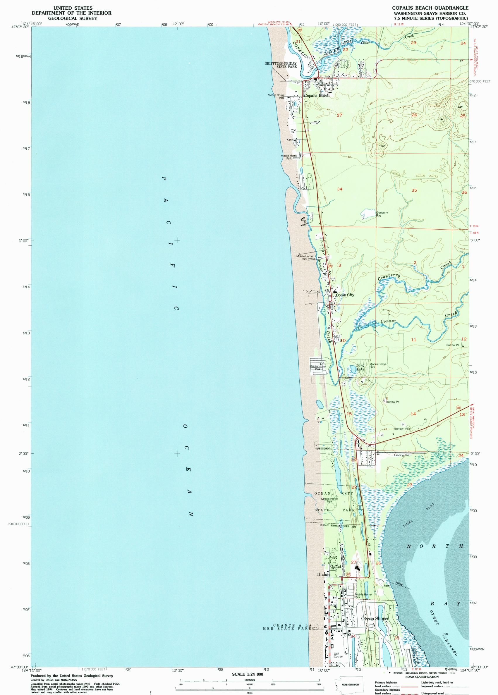
North American Datum of 1927 (NAD 27). Projection and blue 1000-meter ticks: Universal Transverse Mercator, zone 10 10 000-foot ticks: Washington Coordinate System, south zone North American Datum of 1983 (NAD 83) is shown by dashed corner ticks. The values of the shift between NAD 27 and NAD 83 for 7.5-minute intersections are obtainable from National Geodetic Survey NADCON Software There may be private inholdings within the boundaries of the National or State reservations shown on this map
