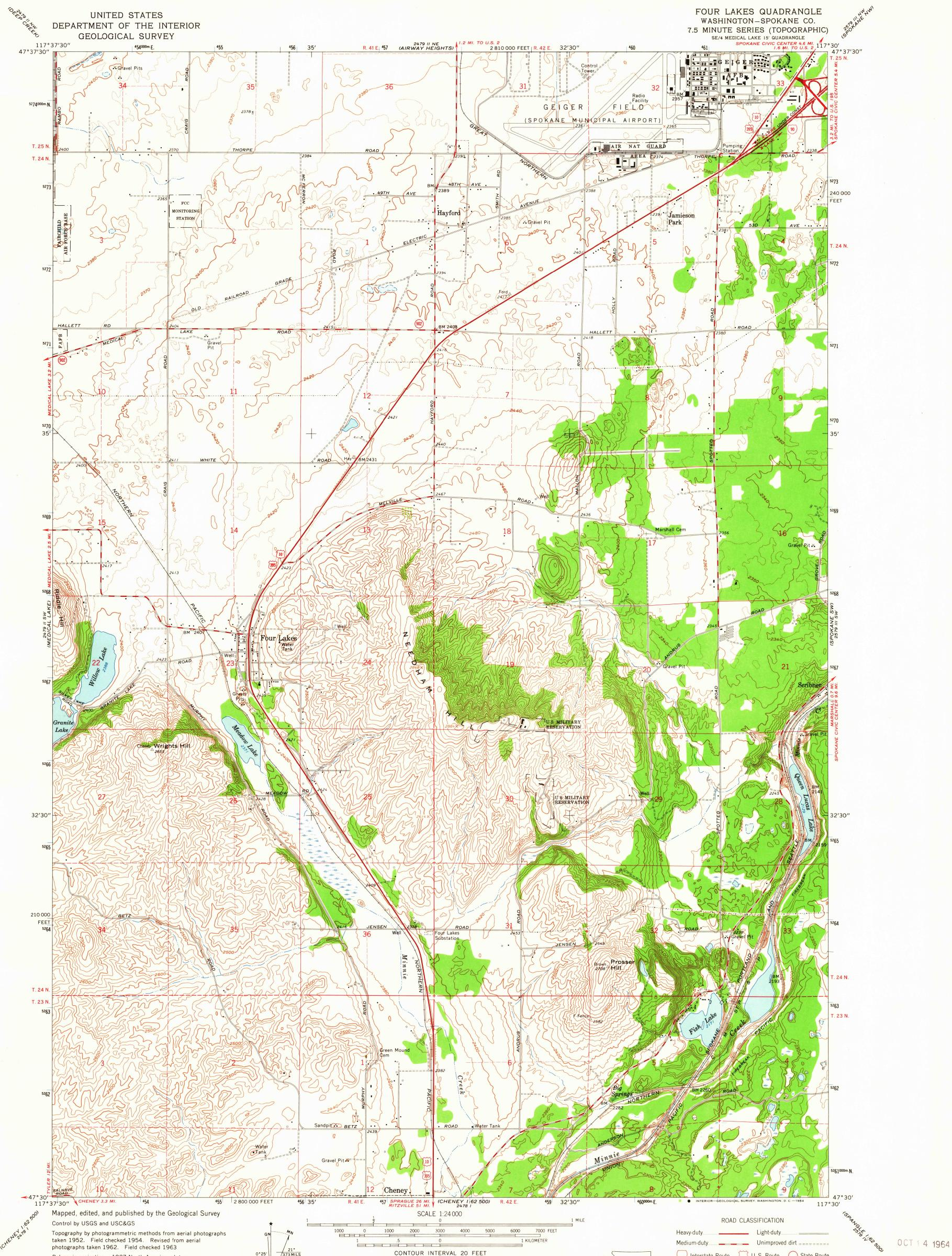
Polyconic projection. 1927 North American datum 10,000-foot grid based on Washington coordinate system, north zone 1000-meter Universal Transverse Mercator grid ticks, zone 11, shown in blue UTM GRID AND 1963 MAGNETIC NORTH DECLINATION AT CENTER OF SHEET
