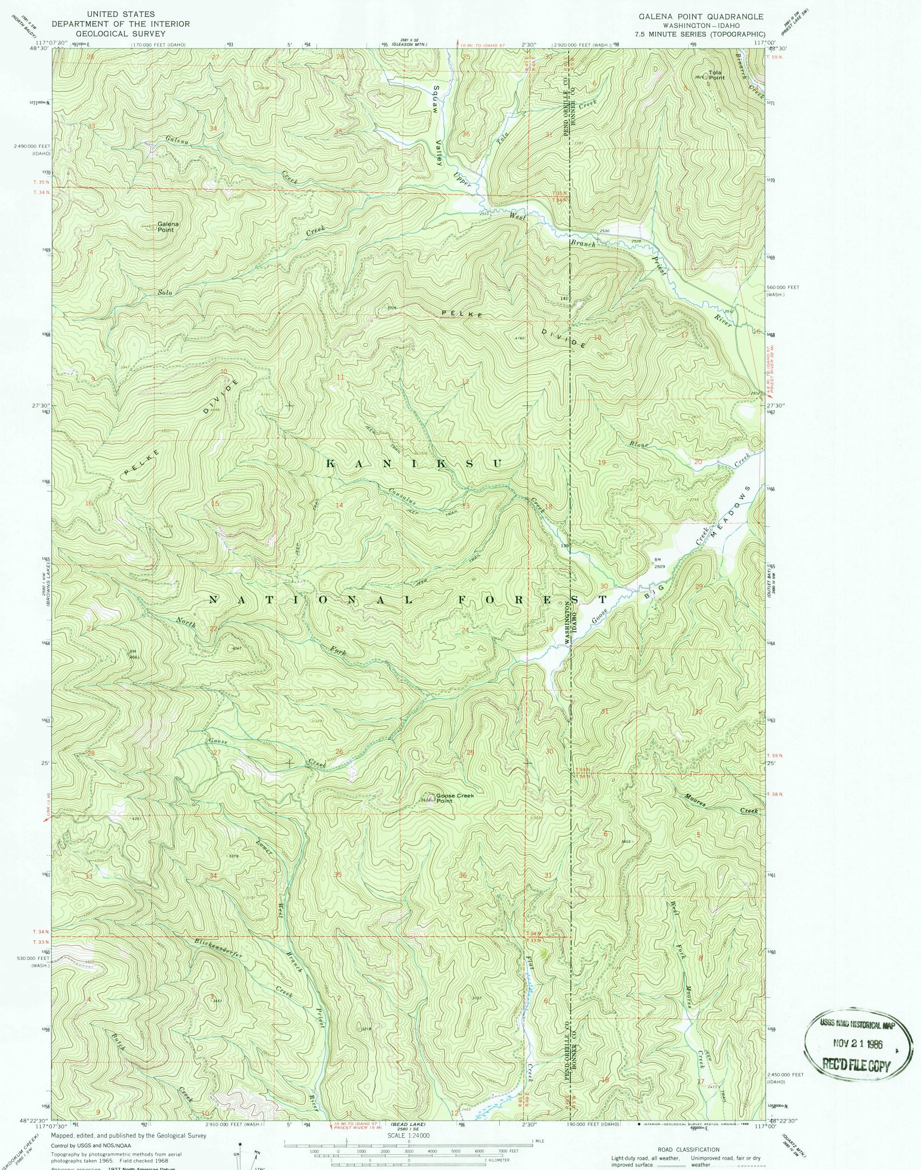
Polyconic projection. 1927 North American Datum 10,000-foot grids based on Washington coordinate system, north zone and Idaho coordinate system, west zone 1000-meter Universal Transverse Mercator grid ticks, zone 11, shown in blue To place on the predicted North American Datum 1983 move the projection lines 14 meters north and 78 meters east as shown by dashed corner ticks There may be private inholdings within the boundaries of the National or State reservations shown on this map
