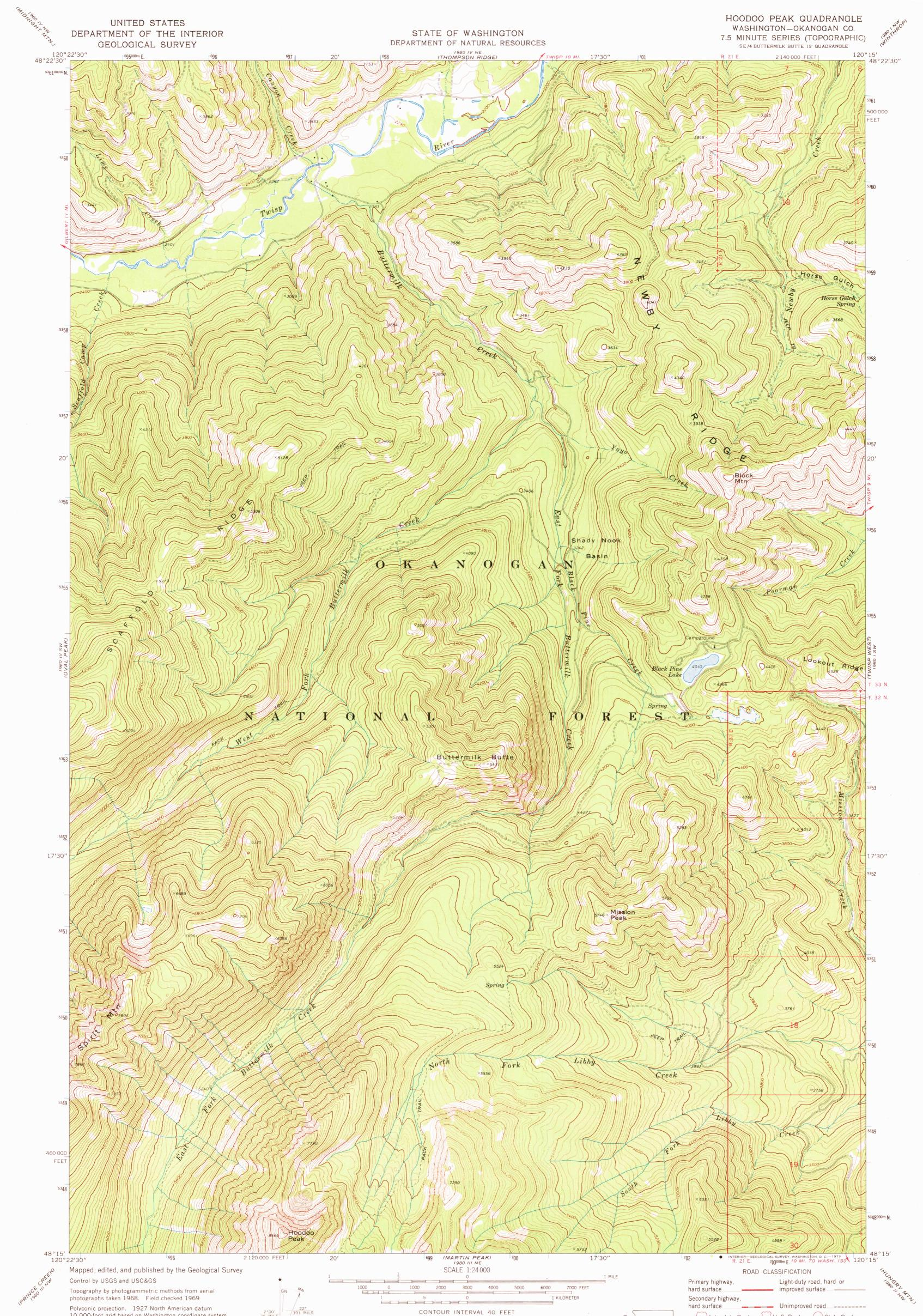
Polyconic projection. 1927 North American datum 2°00' 36 MILS 10,000-foot grid based on Washington coordinate system, north zone 1000-meter Universal Transverse Mercator grid ticks, zone 10, shown in blue UTM GRID AND 1969 MAGNETIC NORTH DECLINATION AT CENTER OF SHEET Where omitted, land lines have not been established
