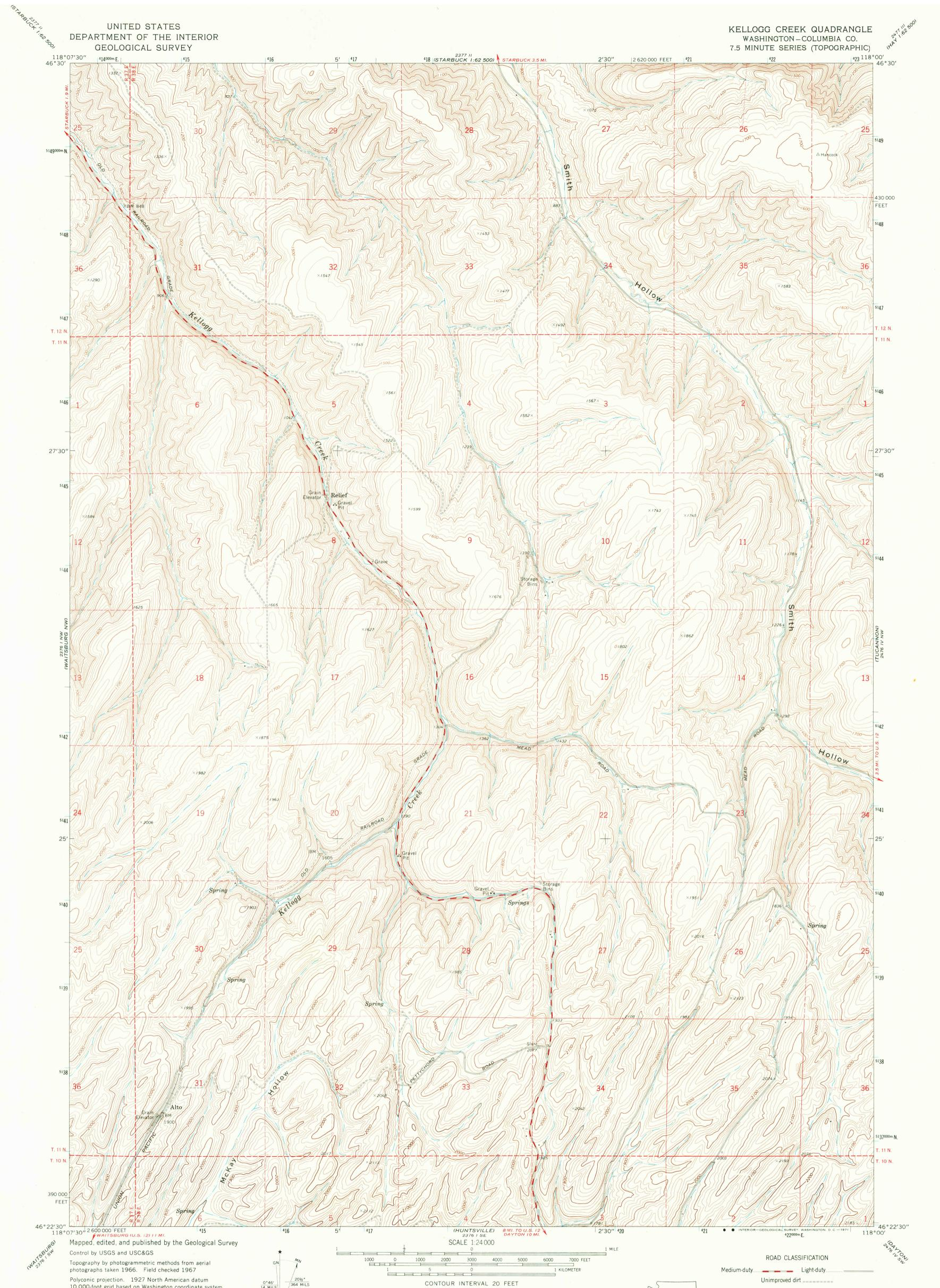
Polyconic projection. 1927 North American datum 0°46' 14 MILS 10,000-foot grid based on Washington coordinate system, south zone 1000-meter Universal Transverse Mercator grid ticks, zone 11, shown in blue UTM GRID AND 1967 MAGNETIC NORTH DECLINATION AT CENTER OF SHEET Fine red dashed lines indicate selected fence lines
