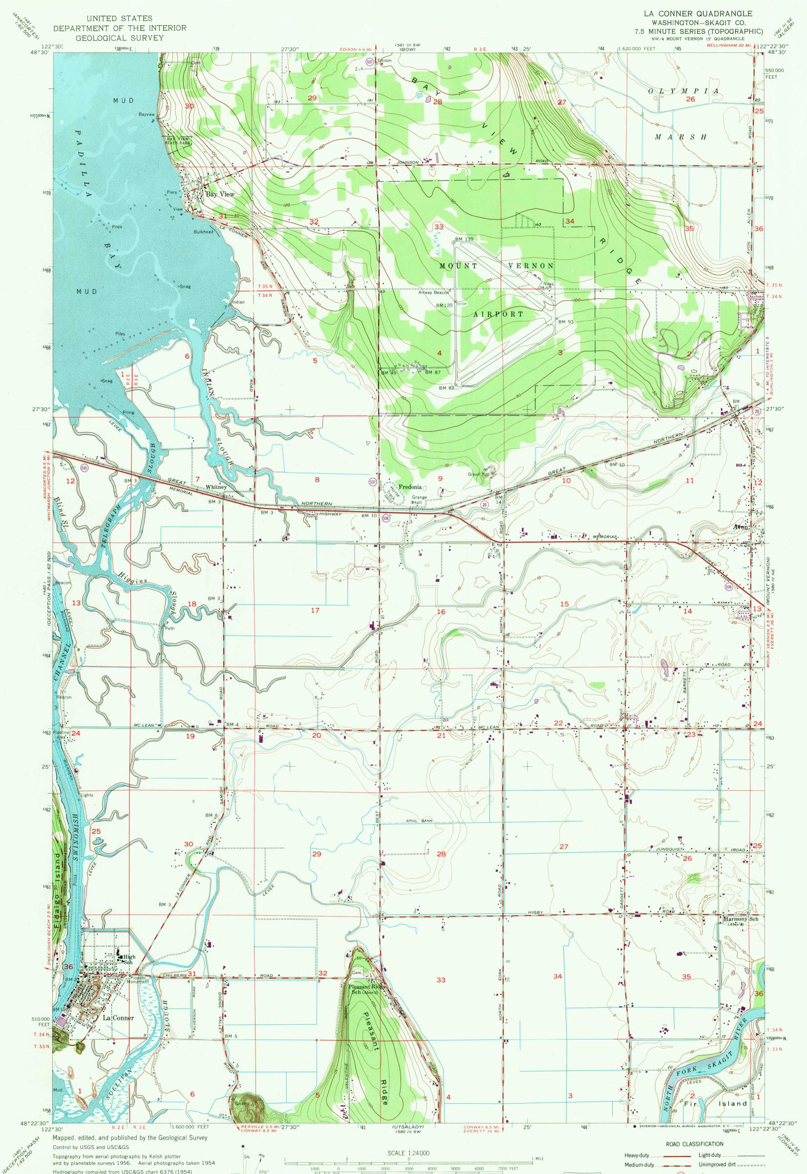
Hydrography compiled from USC&GS chart 6376 (1954) Polyconic projection. 1927 North American datum 10,000-foot grid based on Washington coordinate system, north zone 1000-meter Universal Transverse Mercator grid ticks,
