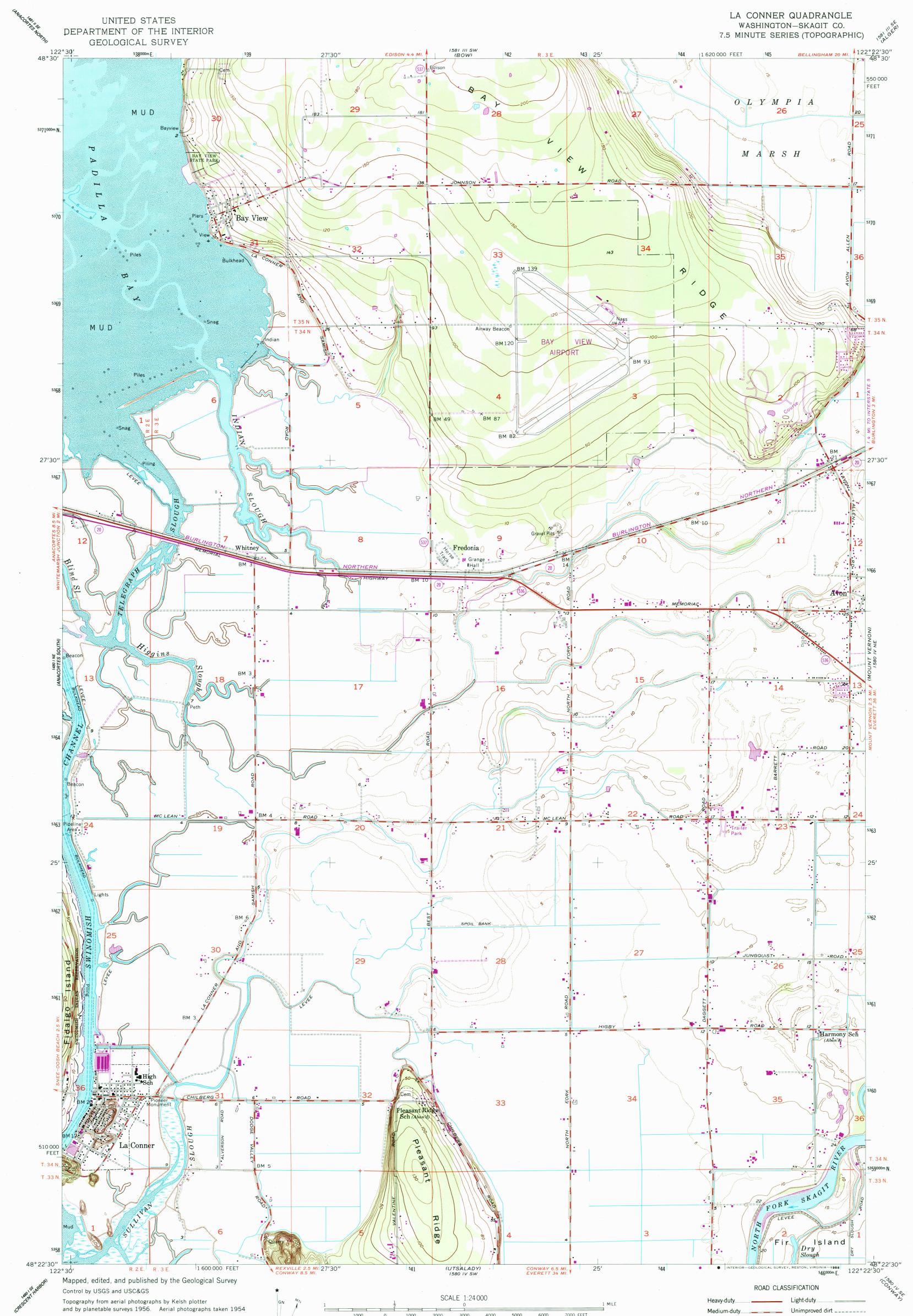
Hydrography compiled from USC&GS chart 6376 (1954) Polyconic projection. 1927 North American datum 10,000-foot grid based on Washington coordinate system, north zone 1000-meter Universal Transverse Mercator grid ticks, zone 10, shown in blue To place on the predicted North American Datum 1983 move the projection lines 23 meters north and 94 meters east as shown by dashed corner ticks
