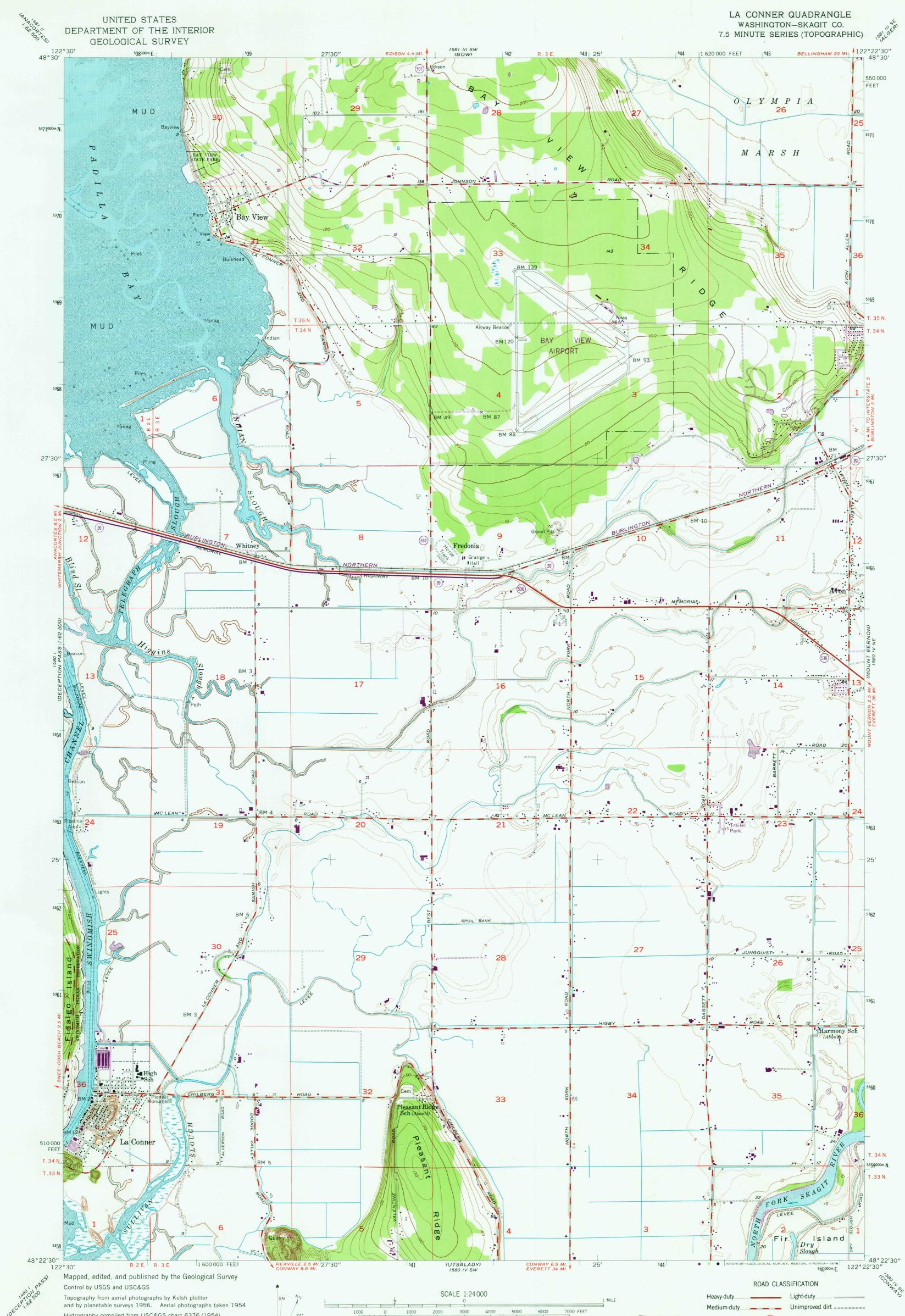
Hydrography compiled from USC&GS chart 6376 (1954) Polyconic projection. 1927 North American datum 10,000-foot grid based on Washington coordinate system, north zone 1000-meter Universal Transverse Mercator grid ticks, UTM GRID AND 1973 MAGNETIC NORTH DECLINATION AT CENTER OF SHEET zone 10, shown in blue
