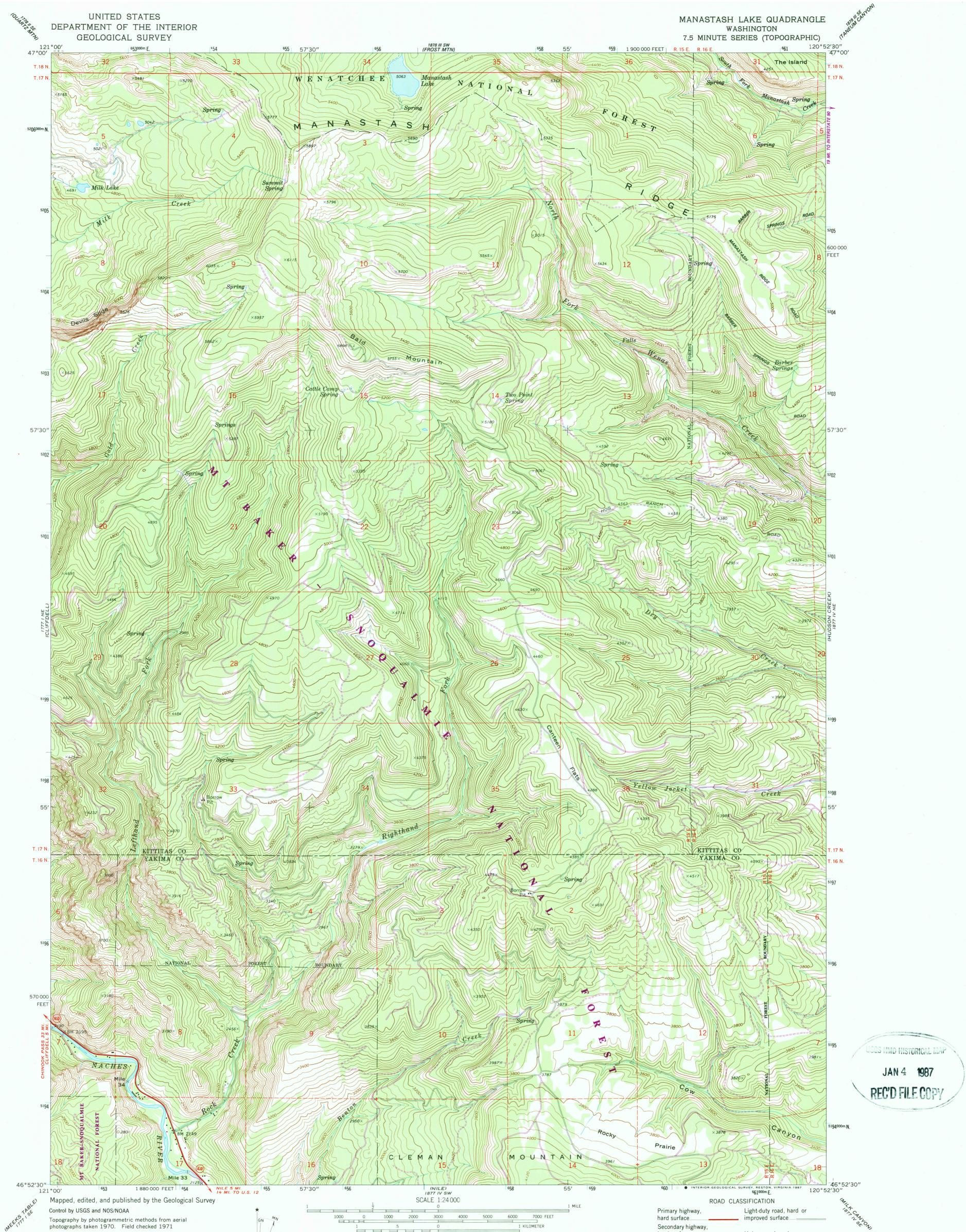
Projection and 10,000-foot grid ticks: Washington coordinate system, south zone (Lambert conformal conic) 1000-meter Universal Transverse Mercator grid ticks, zone 10, shown in blue. 1927 North American Datum
