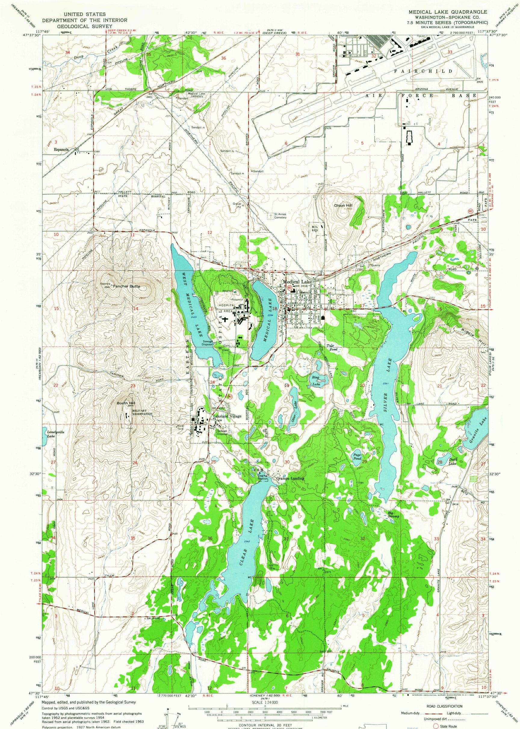
0°30' 9 MILS Polyconic projection. 1927 North American datum 10,000-foot grid based on Washington coordinate system, north zone 1000-meter Universal Transverse Mercator grid ticks, zone 11, shown in blue UTM GRID AND 1963 MAGNETIC NORTH DECLINATION AT CENTER OF SHEET Fine red dashed lines indicate selected fence lines
