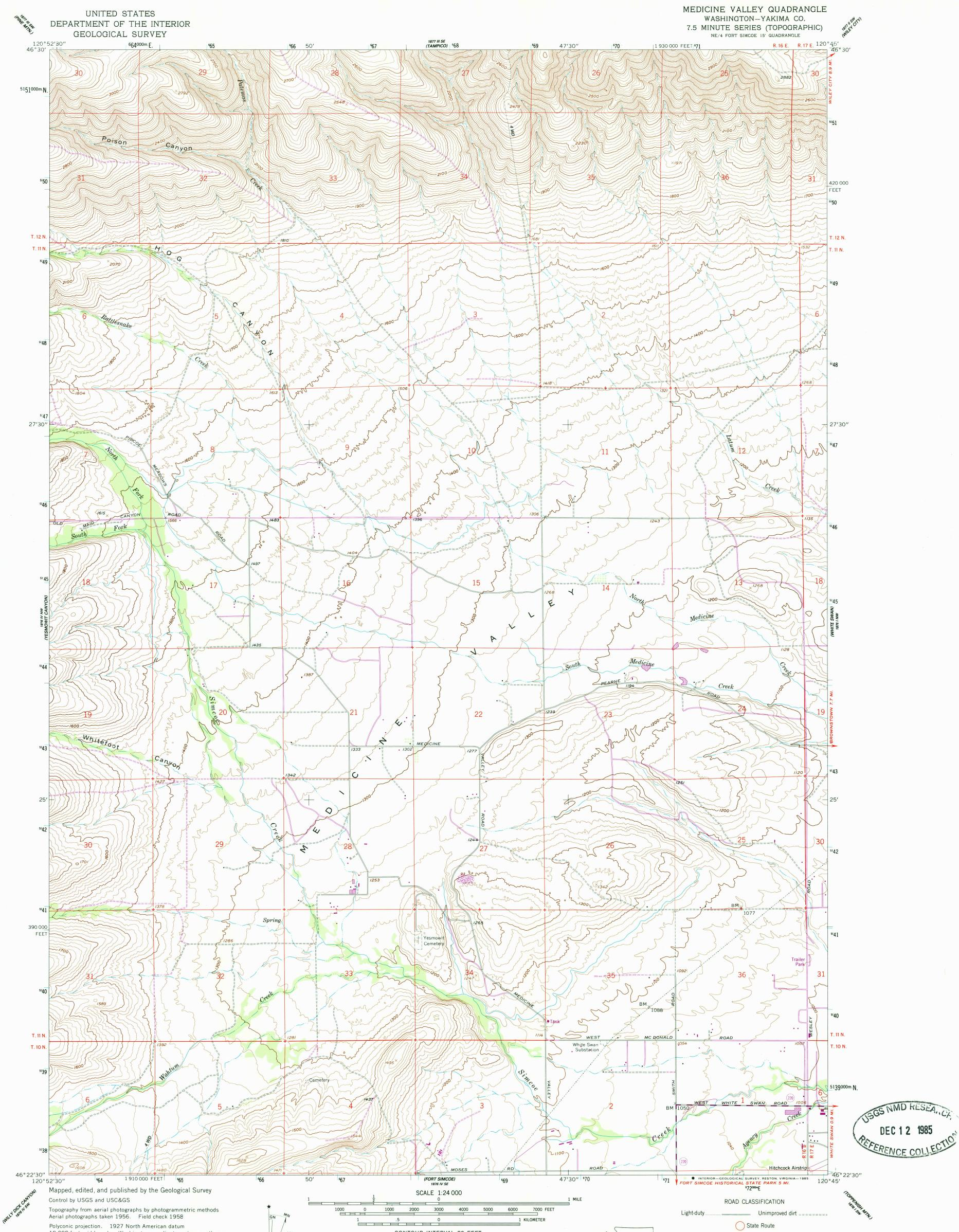
Polyconic projection. 1927 North American datum 10,000-foot grid based on Washington coordinate system, south zone 1000-meter Universal Transverse Mercator grid ticks, zone 10, shown in blue
