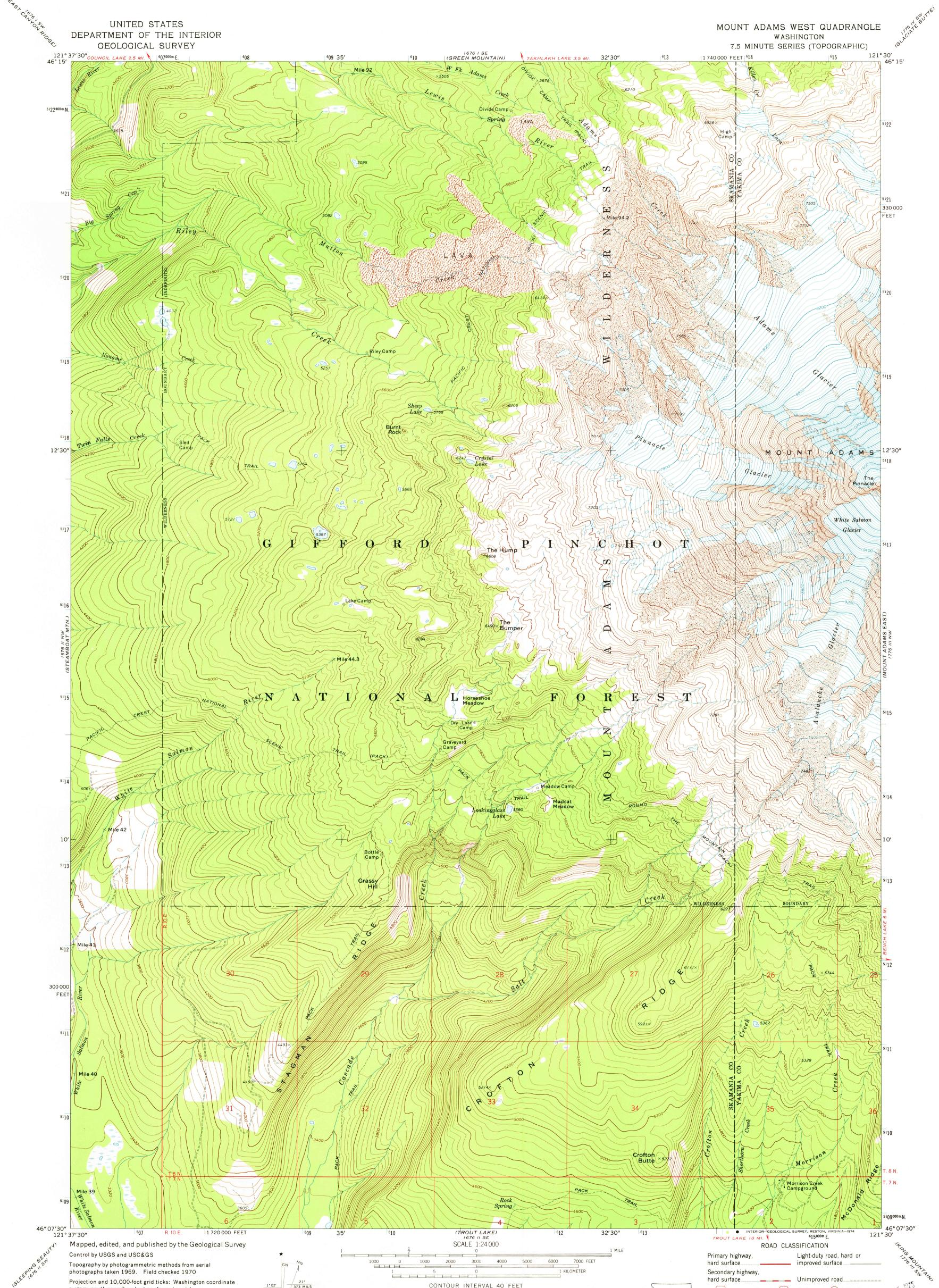
Projection and 10,000-foot grid ticks: Washington coordinate system, south zone (Lambert conformal conic) 1000-meter Universal Transverse Mercator grid ticks, zone 10, shown in blue. 1927 North American datum
