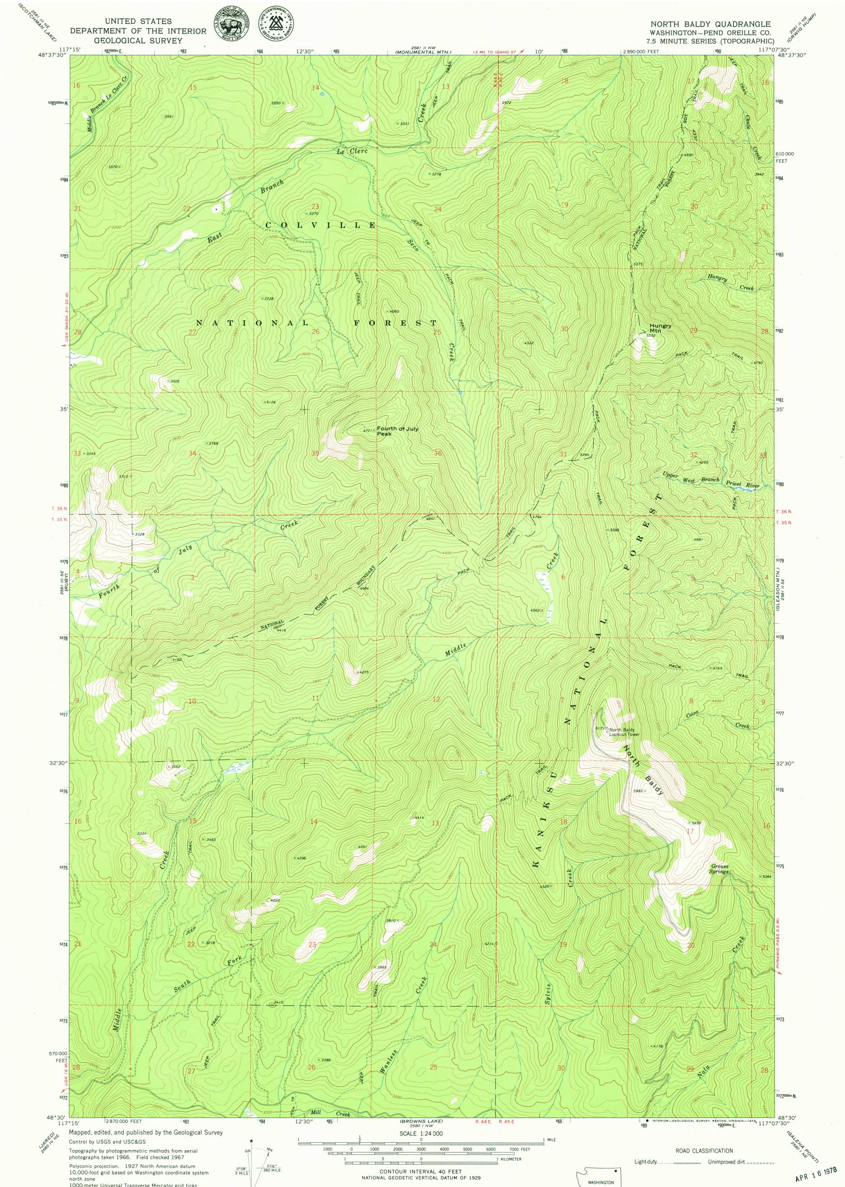
Polyconic projection. 1927 North American datum 10,000-foot grid based on Washington coordinate system north zone 1000-meter Universal Transverse Mercator grid ticks, zone 11, shown in blue
