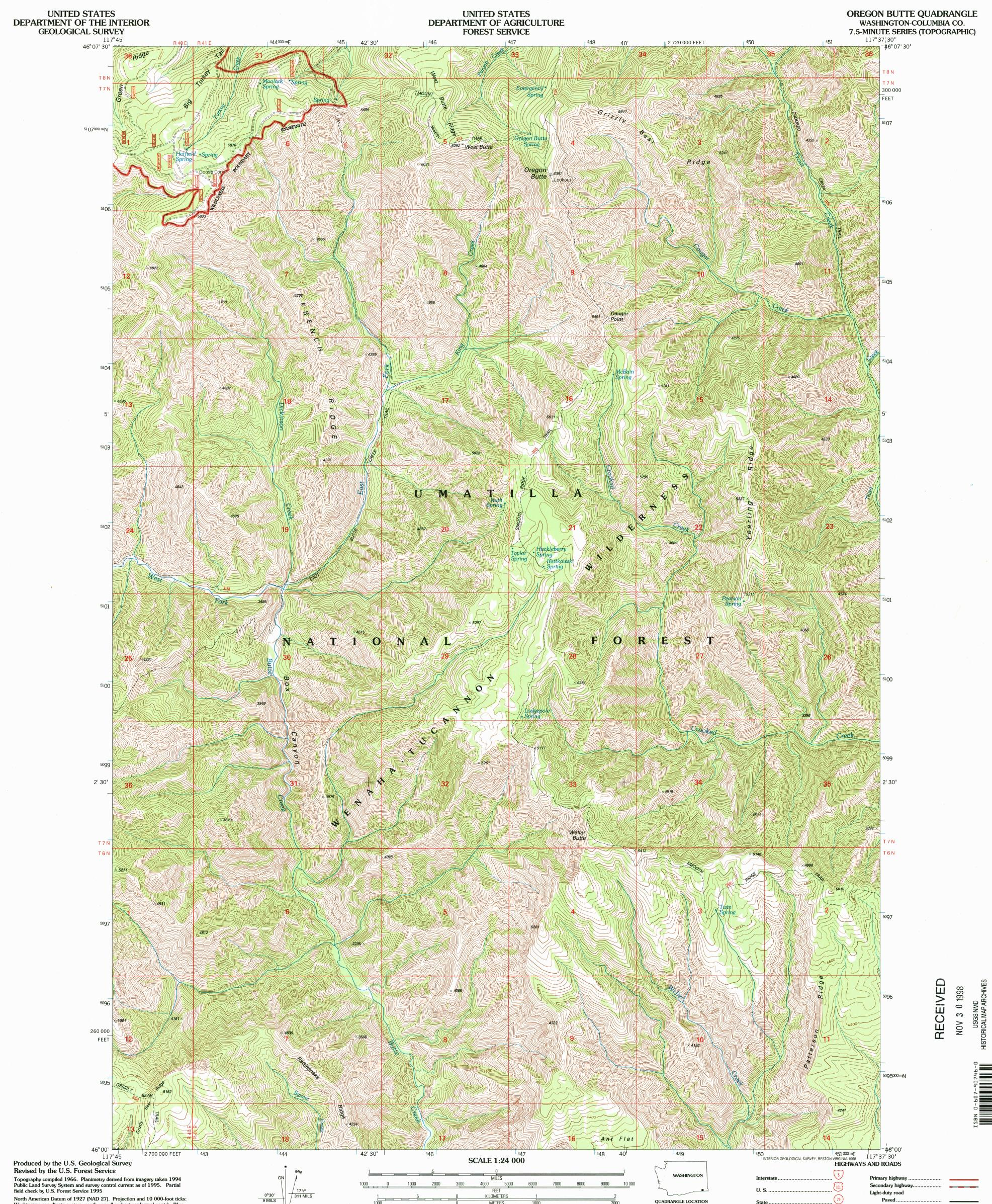
North American Datum of 1927 (NAD 27). Projection and 10 000-foot ticks: Washington coordinate system, south zone (Lambert conformal conic). Blue 1000-meter Universal Transverse Mercator ticks, zone 11
