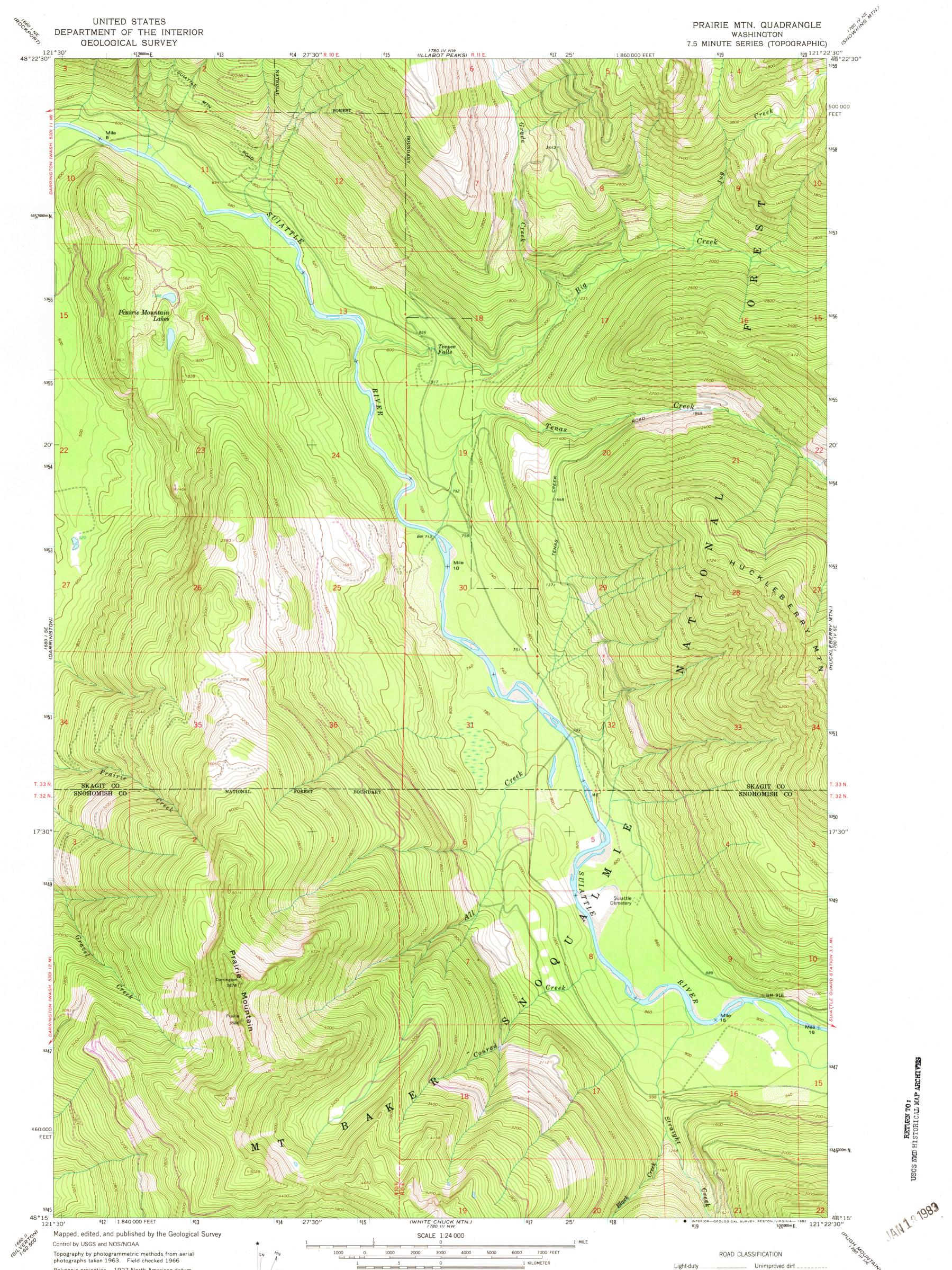
Polyconic projection. 1927 North American datum 10,000-foot grid based on Washington coordinate system, north zone 1000-meter Universal Transverse Mercator grid ticks, zone 10, shown in blue To place on the predicted North American Datum 1983 move the projection lines 22 meters north and 91 meters east as shown by dashed corner ticks Where omitted, land lines have not been established There may be private inholdings within the boundaries of the National or State reservations shown on this map
