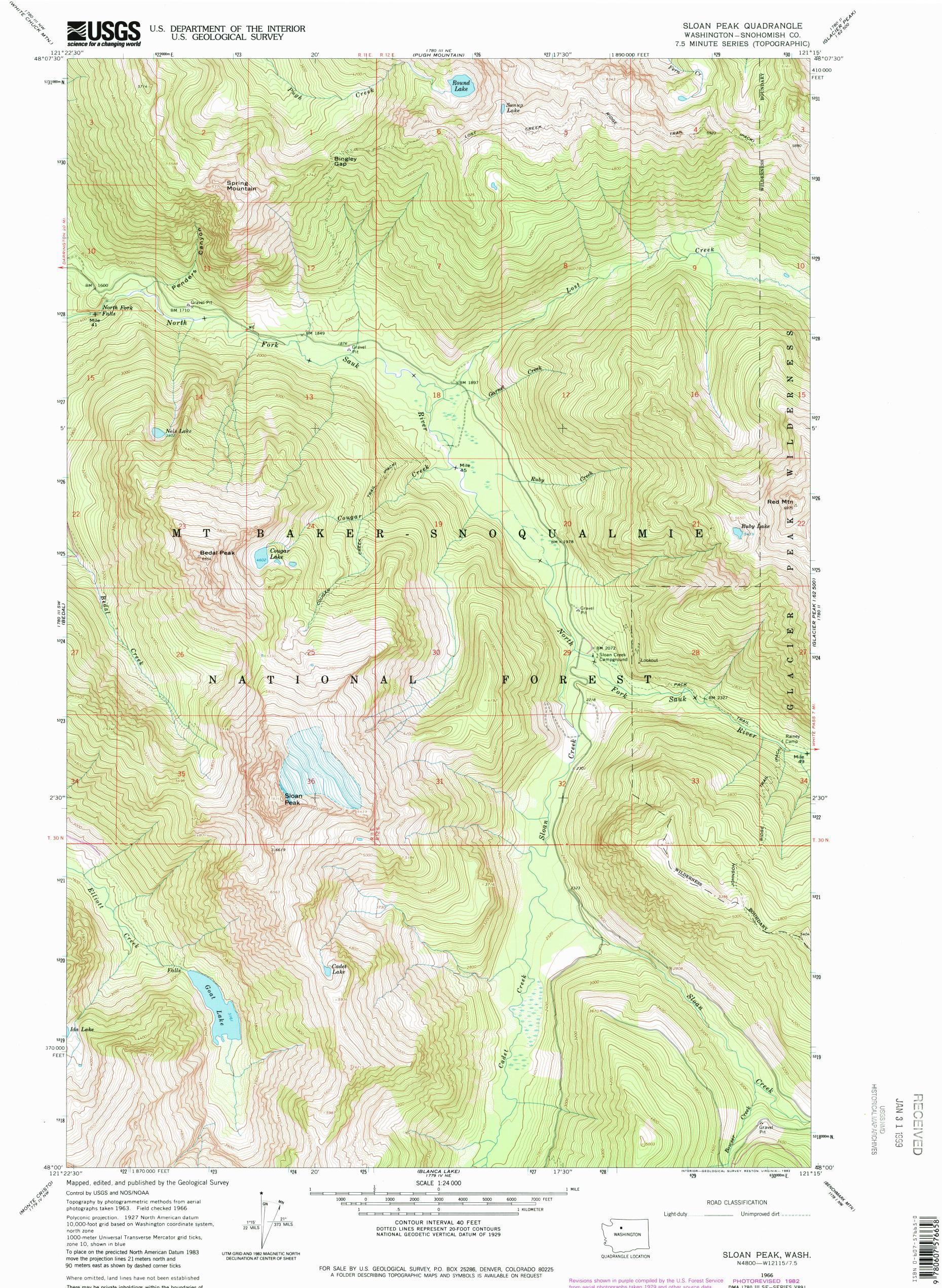
Polyconic projection. 1927 North American datum 1°15' 22 MILS 10,000-foot grid based on Washington coordinate system, north zone 1000-meter Universal Transverse Mercator grid ticks, zone 10, shown in blue To place on the predicted North American Datum 1983 UTM GRID AND 1982 MAGNETIC NORTH DECLINATION AT CENTER OF SHEET move the projection lines 21 meters north and 90 meters east as shown by dashed corner ticks
