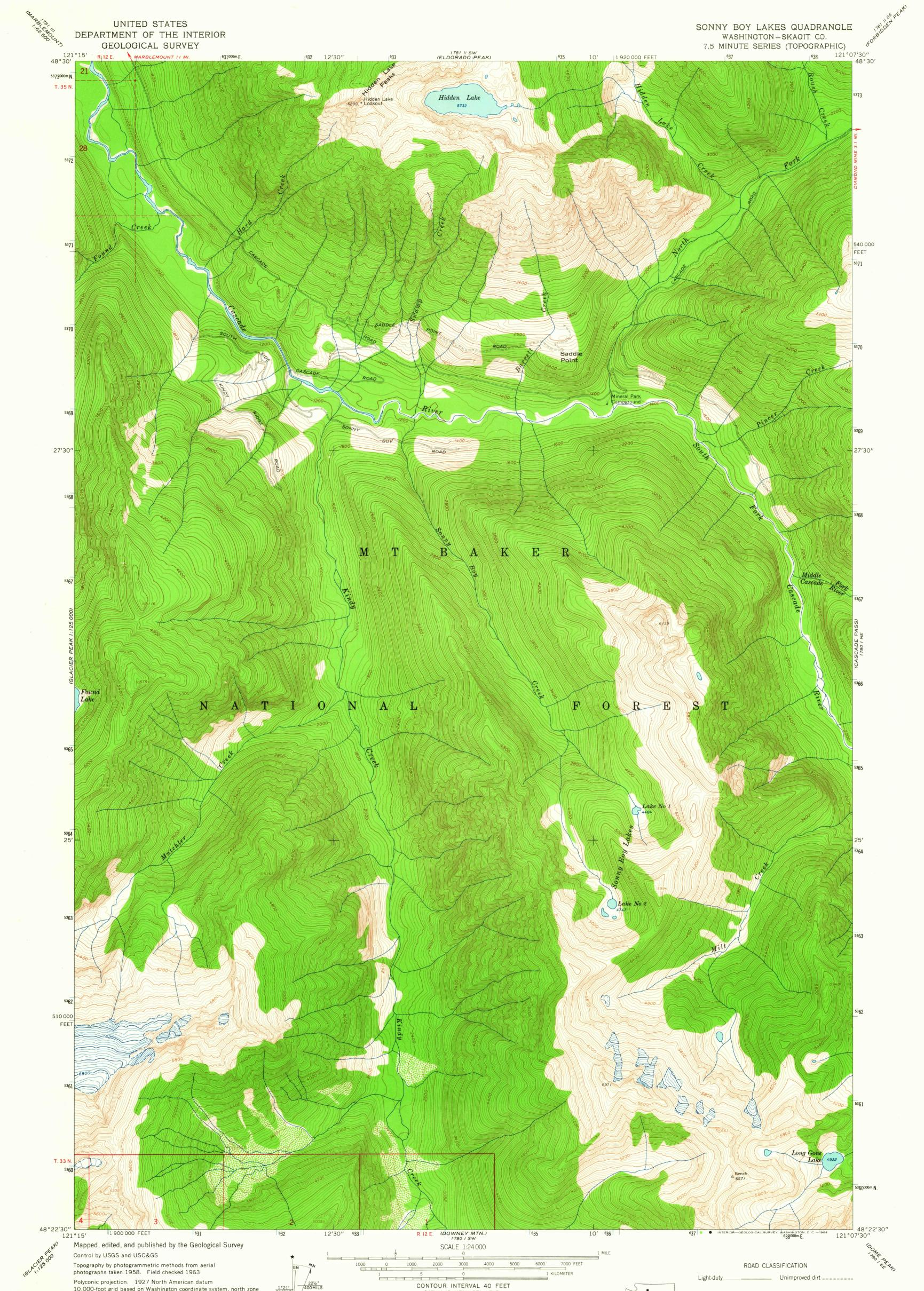
Polyconic projection. 1927 North American datum 1°21′ 24 MILS 10,000-foot grid based on Washington coordinate system, north zone 1000-meter Universal Transverse Mercator grid ticks, zone 10, shown in blue
