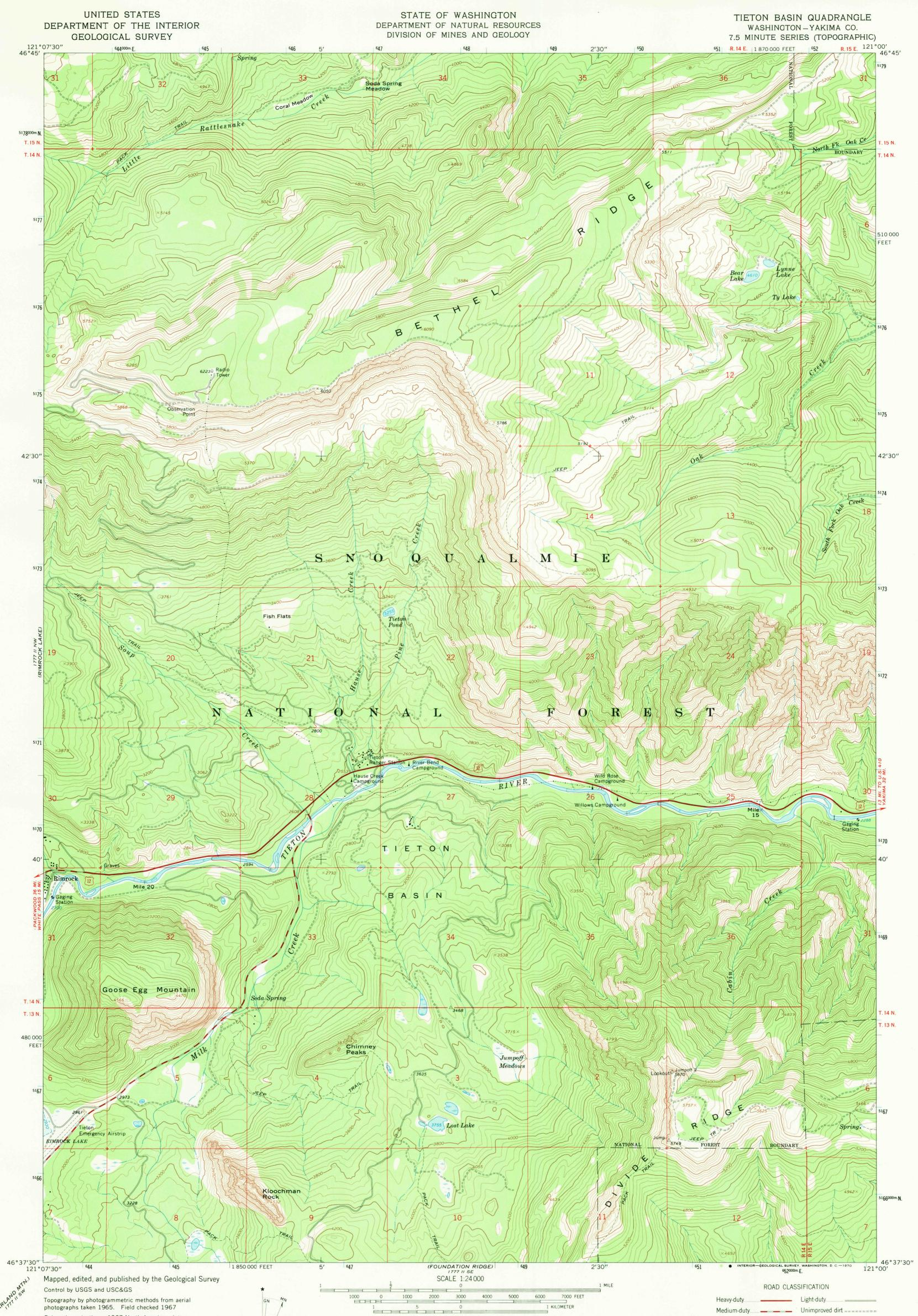
Polyconic projection. 1927 North American datum 10,000-foot grid based on Washington coordinate system, south zone 1000-meter Universal Transverse Mercator grid ticks, zone 10, shown in blue Where omitted, land lines have not been established Areas covered by dashed light-blue pattern are subject to controlled inundation Horizon AT CENTER OF SHEET
