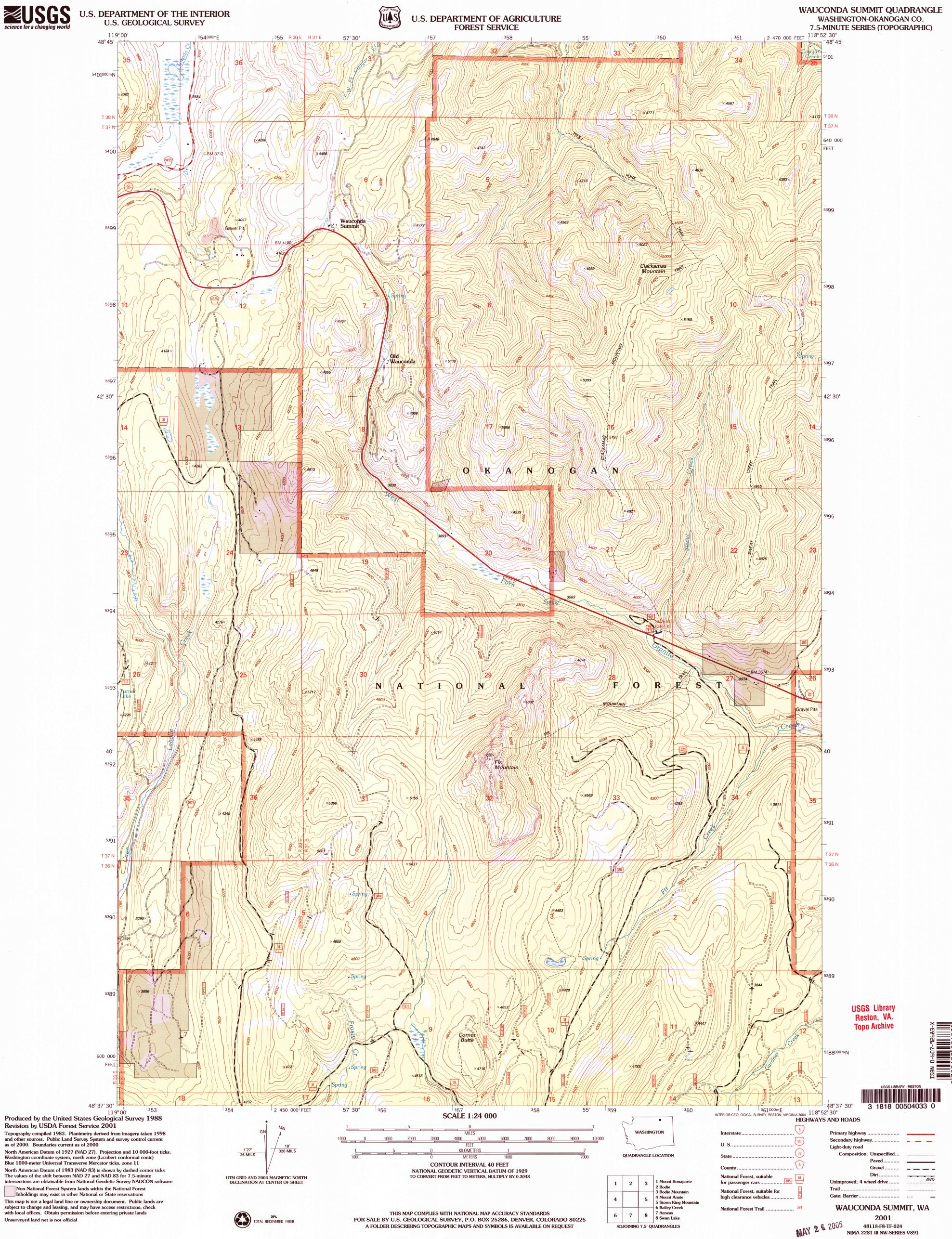
Blue 1000-meter Universal Transverse Mercator ticks, zone 11 North American Datum of 1983 (NAD 83) is shown by dashed corner ticks The values of the shift between NAD 27 and NAD 83 for 7.5-minute intersections are obtainable from National Geodetic Survey NADCON software
