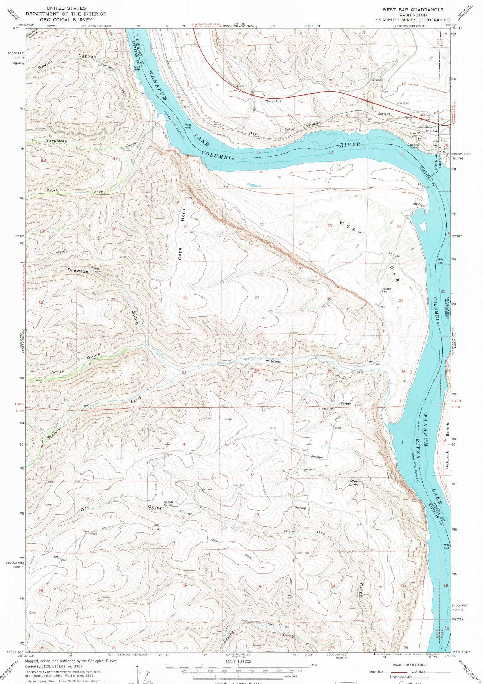
Polyconic projection. 1927 North American datum 21½° 382 MILS 2°09' 38 MILS 10,000-foot grids based on Washington coordinate system, south and north zones 1000-meter Universal Transverse Mercator grid ticks, zone 10, shown in blue UTM GRID AND 1966 MAGNETIC NORTH DECLINATION AT CENTER OF SHEET To place on the predicted North American Datum 1983 move the projection lines 20 meters north and 88 meters east as shown by dashed corner ticks
