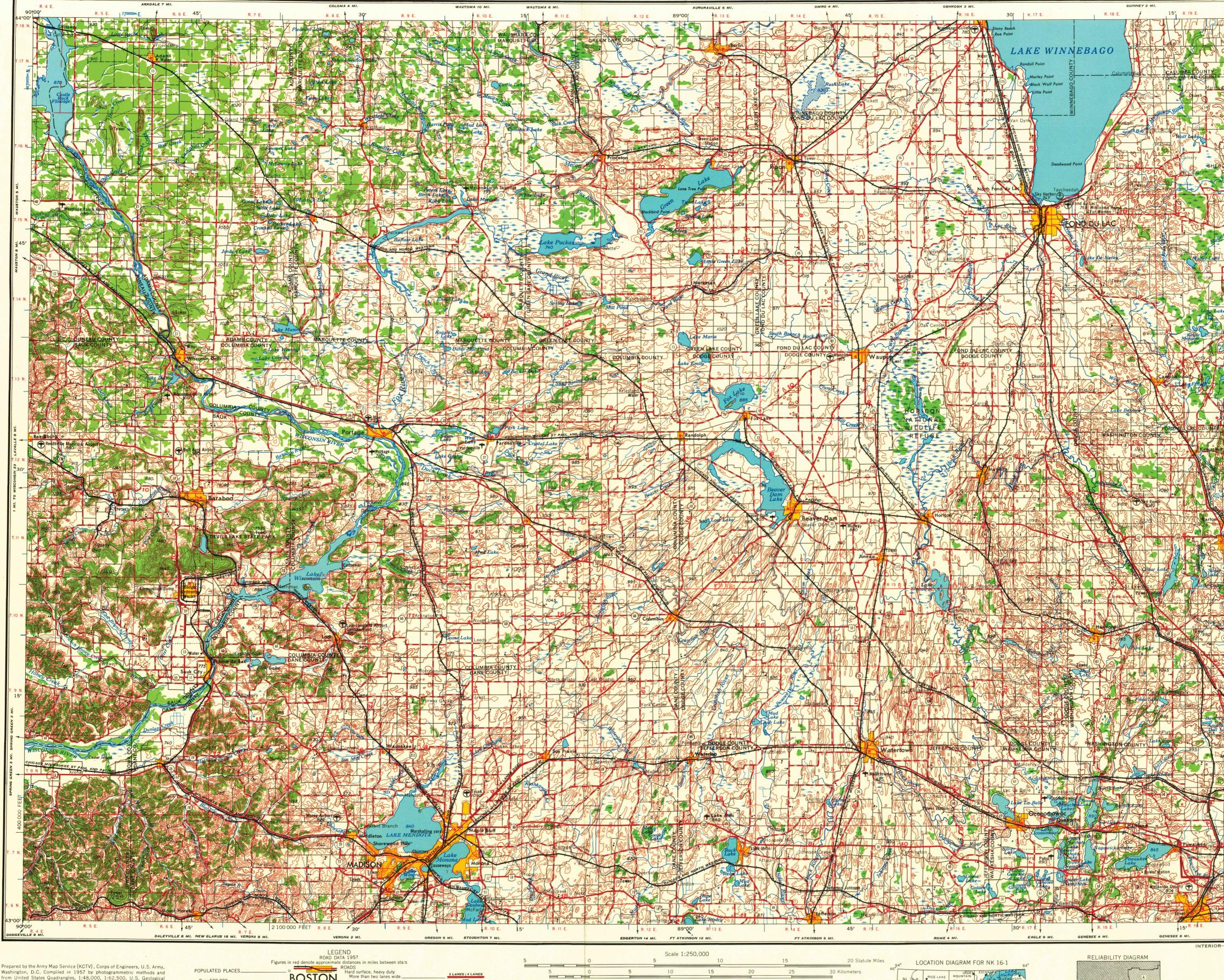
Prepared by the Army Map Service (KCTV), Corps of Engineers, U.S. Army, Washington, D.C. Compiled in 1957 by photogrammetric methods and from United States Quadrangles, 1:48,000, 1:62,500, U.S. Geological Survey, 1954-55. Control by USC&GS and USGS. Map field checked 1957. 100,000-foot grid based on Wisconsin coordinate system, south zone
