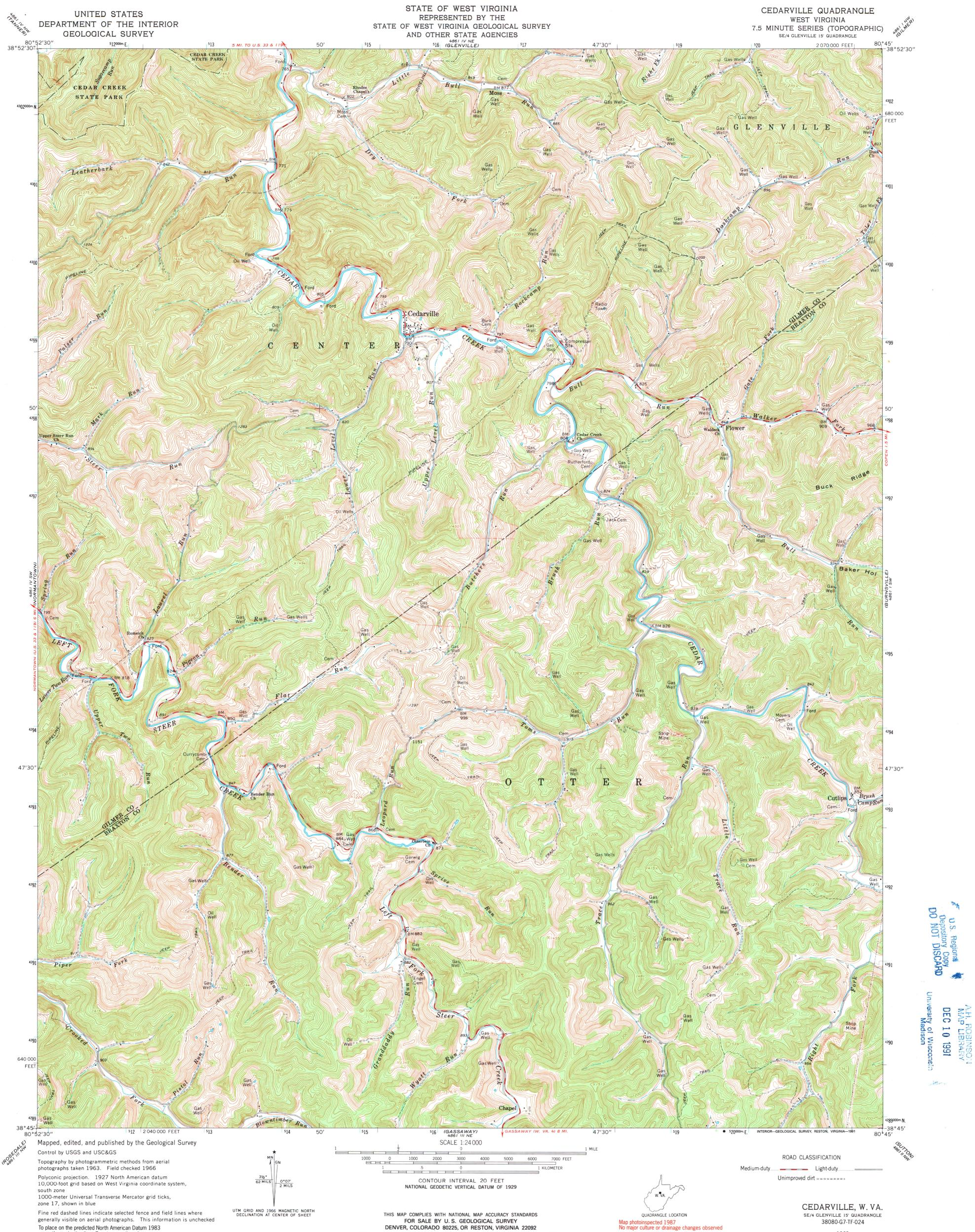
To place on the predicted North American Datum 1983 move the projection lines 7 meters south and 16 meters west as shown by dashed corner ticks
