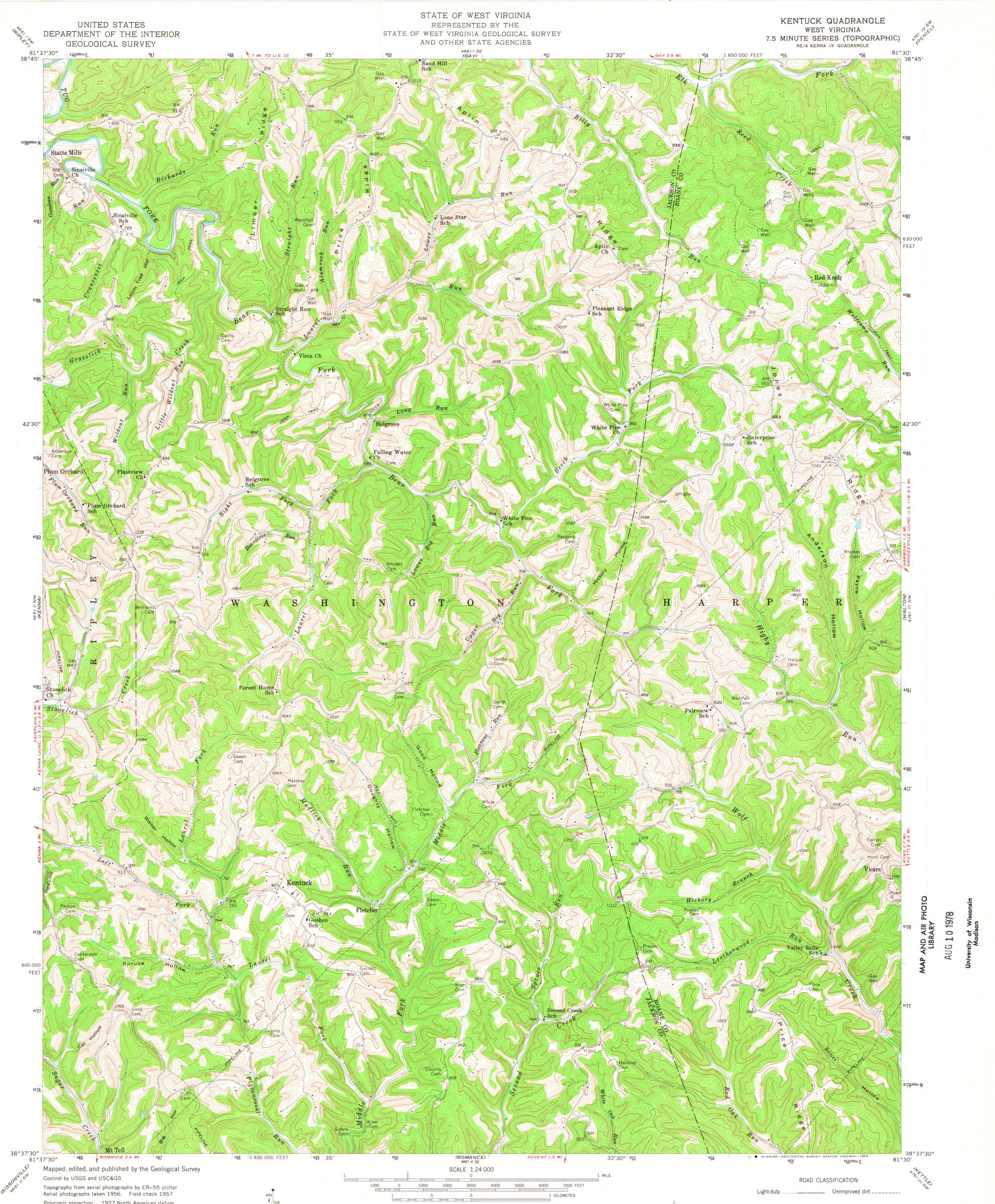
Polyconic projection. 1927 North American datum 10,000-foot grid based on West Virginia coordinate system, south zone 1000-meter Universal Transverse Mercator grid ticks, zone 17, shown in blue
