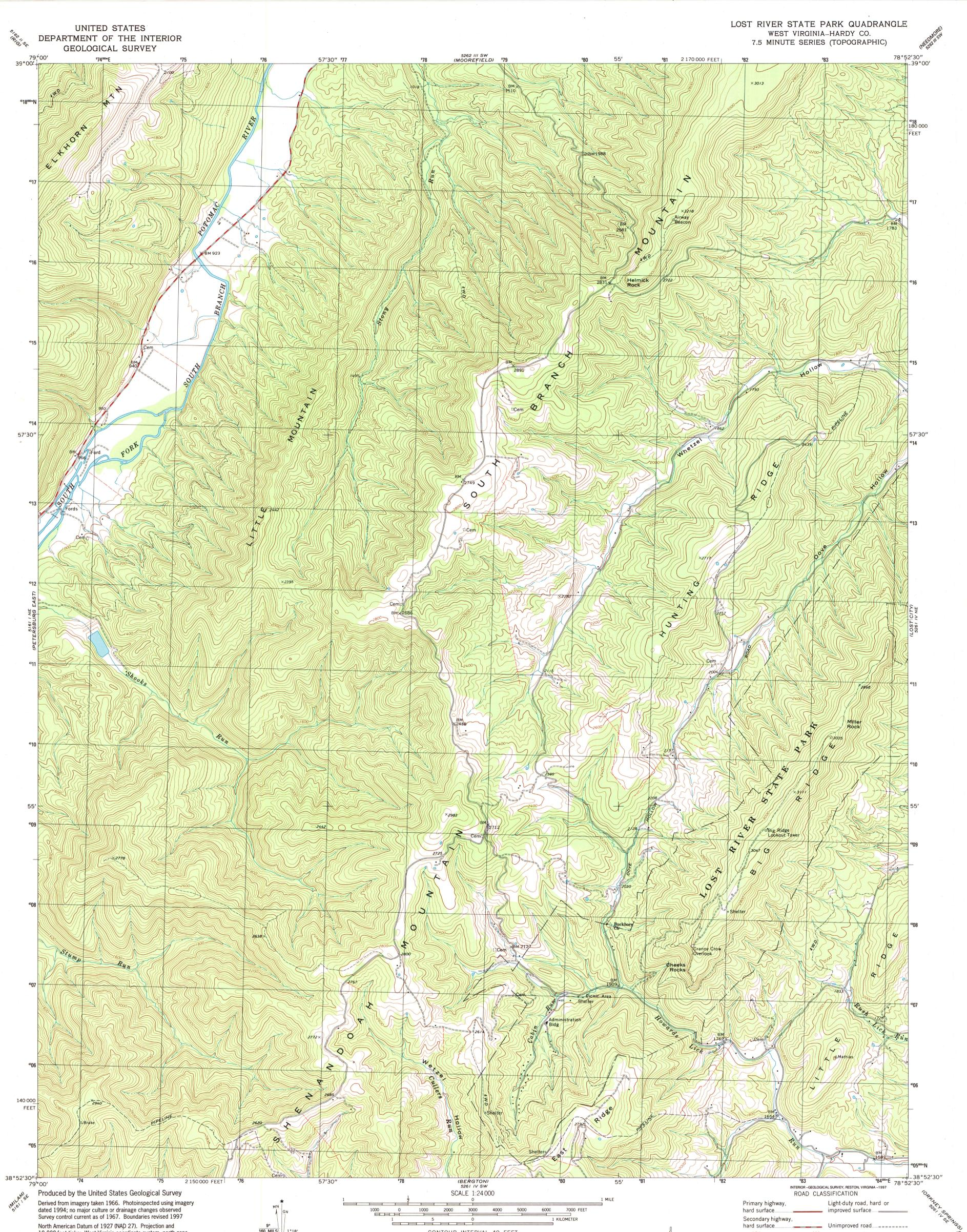
North American Datum of 1927 (NAD 27). Projection and 10 000-foot ticks: West Virginia coordinate system, north zone (Lambert conformal conic) 1000-meter Universal Transverse Mercator grid, zone 17
