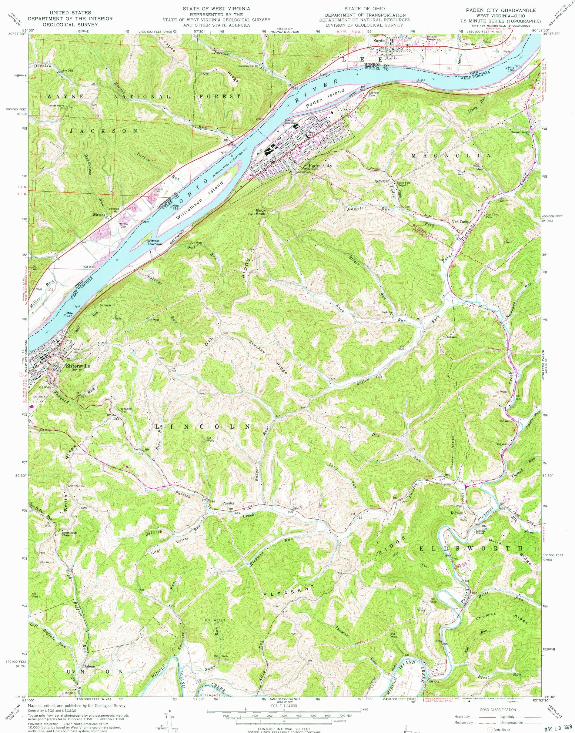
Polyconic projection. 1927 North American datum 10,000-foot grids based on West Virginia coordinate system, north zone, and Ohio coordinate system, south zone 1000-meter Universal Transverse Mercator grid ticks, zone 17, shown in blue
