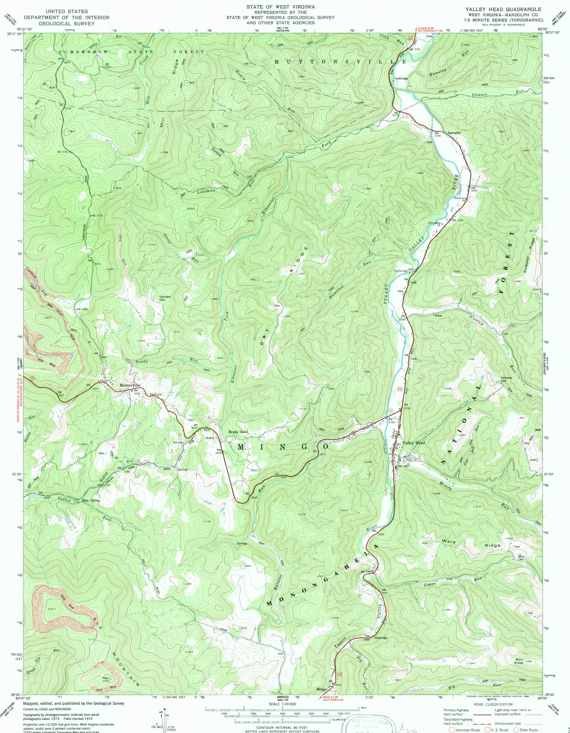
1000-meter Universal Transverse Mercator grid ticks, zone 17, shown in blue 1927 North American Datum To place on the predicted North American Datum 1983 move the projection lines 8 meters south and 19 meters west as shown by dashed corner ticks
