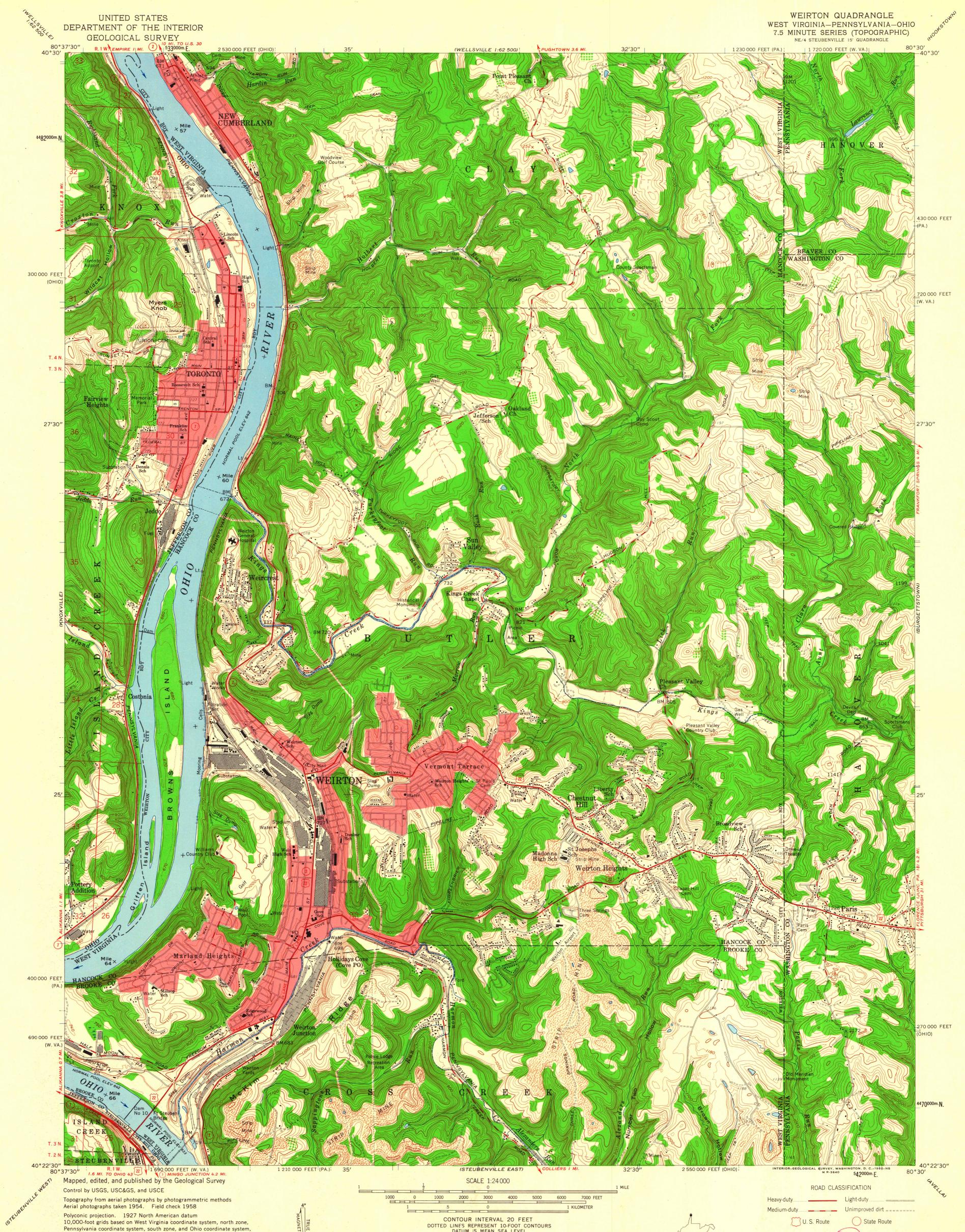
Polyconic projection. 1927 North American datum 10,000-foot grids based on West Virginia coordinate system, north zone, Pennsylvania coordinate system, south zone, and Ohio coordinate system, north zone. 1000-meter Universal Transverse Mercator grid ticks, zone 17, shown in blue
